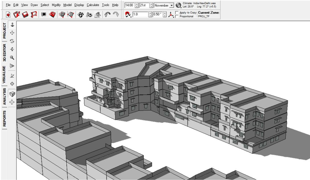
FIGURE 123: SHADOW RANGE ON 21<sup>ST</sup> NOVEMBER 2 PM WITHOUT VIADUCT
