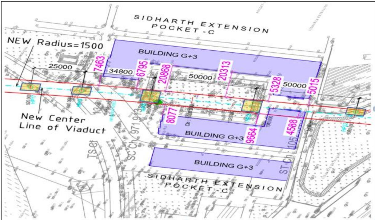
Figure 2: Plan Showing Alignment of Siddharth Extension-Old Alignment
