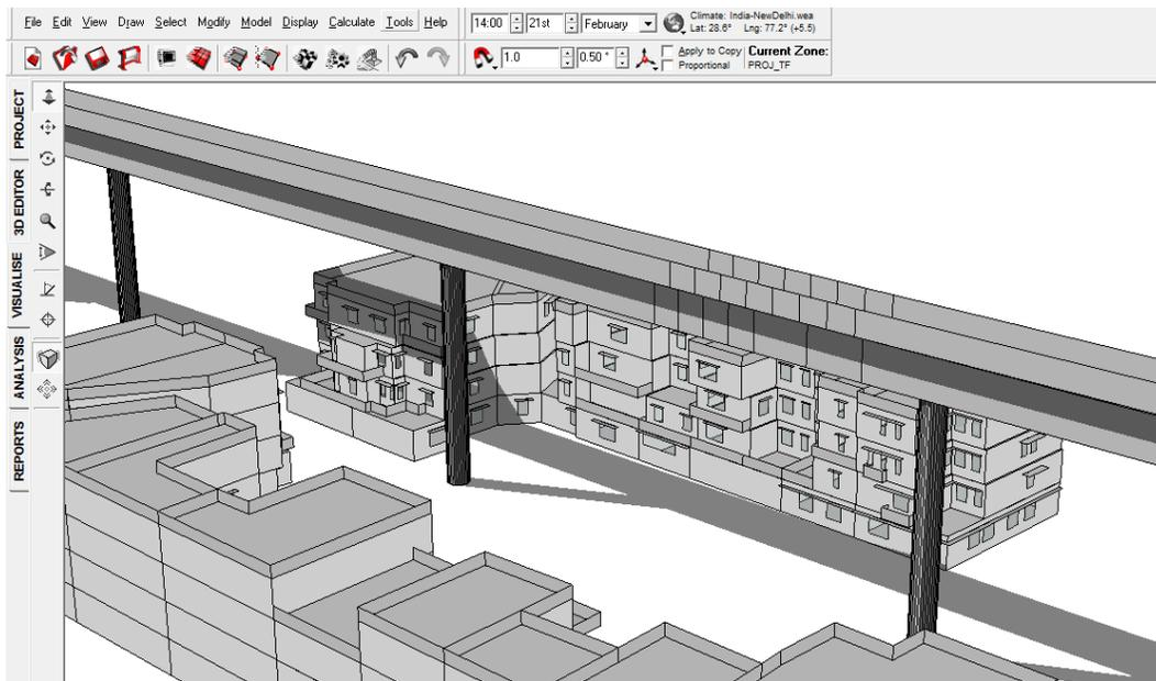
FIGURE 106: SHADOW RANGE ON 21<sup>ST</sup> FEBRUARY 2 PM WITH VIADUCT
