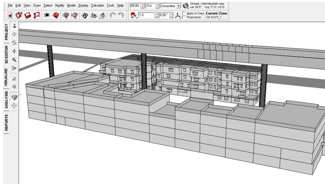
FIGURE 18: SHADOW RANGE ON 21<sup>ST</sup> DECEMBER 9 AM WITH VIADUCT
