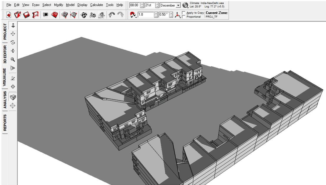
FIGURE 9: SHADOW RANGE ON 21<sup>ST</sup> DECEMBER 8 AM WITHOUT VIADUCT
