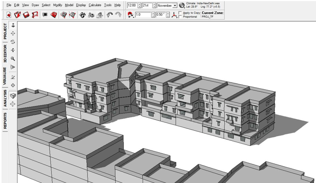
FIGURE 75: SHADOW RANGE ON 21<sup>ST</sup> NOVEMBER 12 PM WITHOUT VIADUCT
