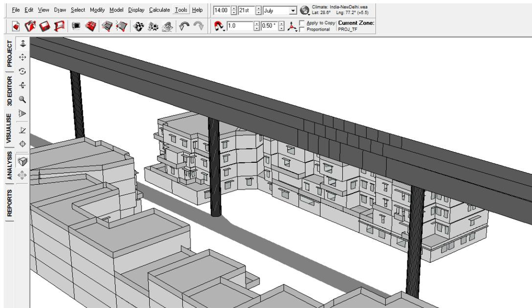
FIGURE 116: SHADOW RANGE ON 21<sup>ST</sup> JULY 2 PM WITH VIADUCT
