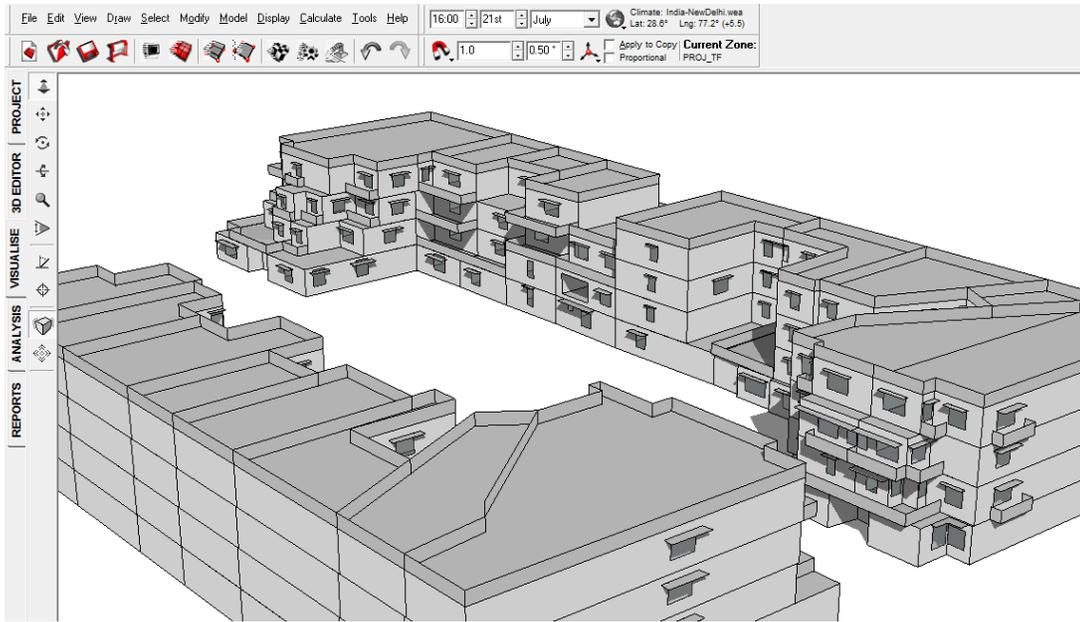
FIGURE 163: SHADOW RANGE ON 21<sup>ST</sup> JULY 4 PM WITHOUT VIADUCT
