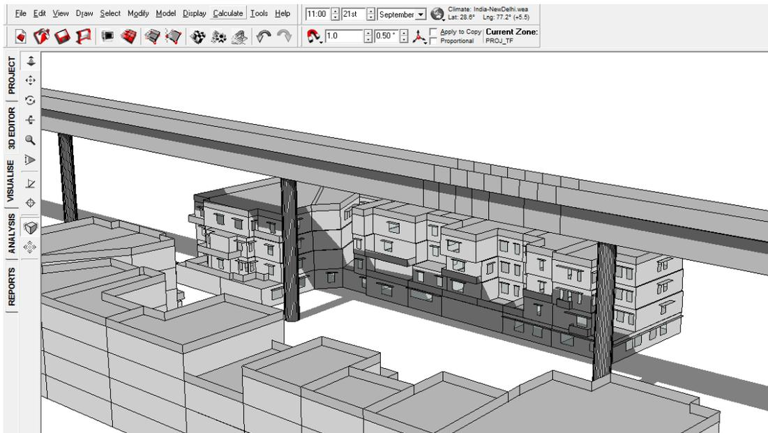
FIGURE 48: SHADOW RANGE ON 21<sup>ST</sup> SEPTEMBER 11 AM WITH VIADUCT
