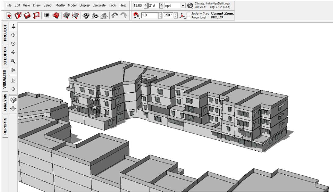
FIGURE 61: SHADOW RANGE ON 21<sup>ST</sup> APRIL 12 PM WITHOUT VIADUCT
