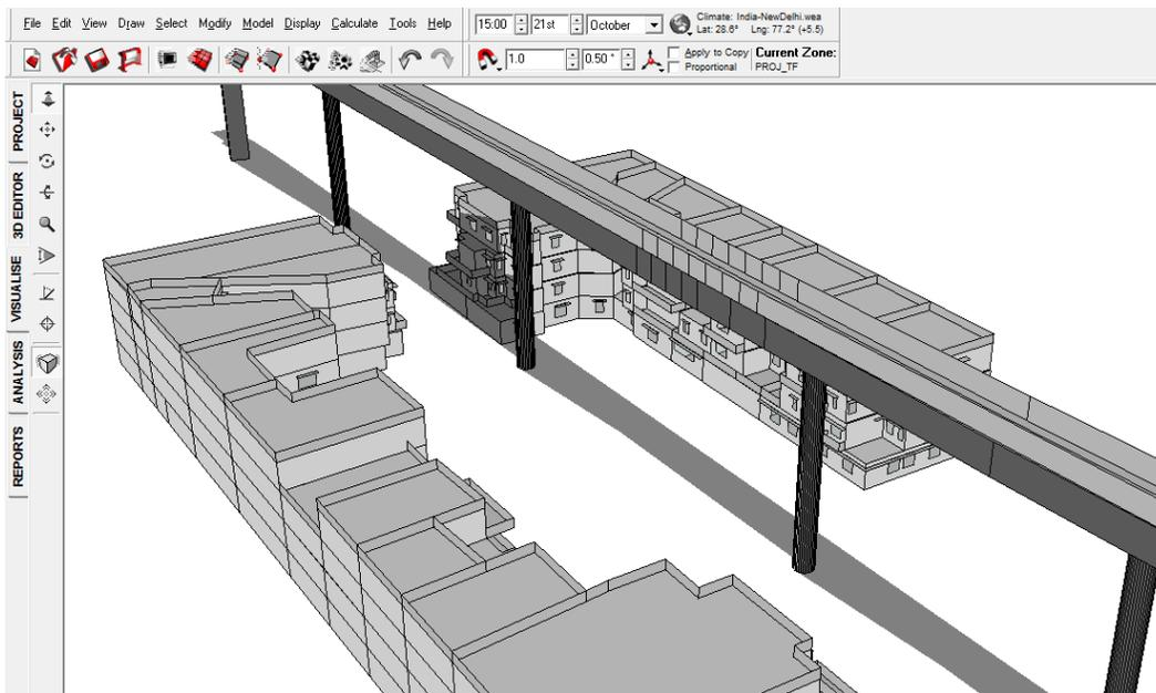
FIGURE 146: SHADOW RANGE ON 21<sup>ST</sup> OCTOBER 3 PM WITH VIADUCT
