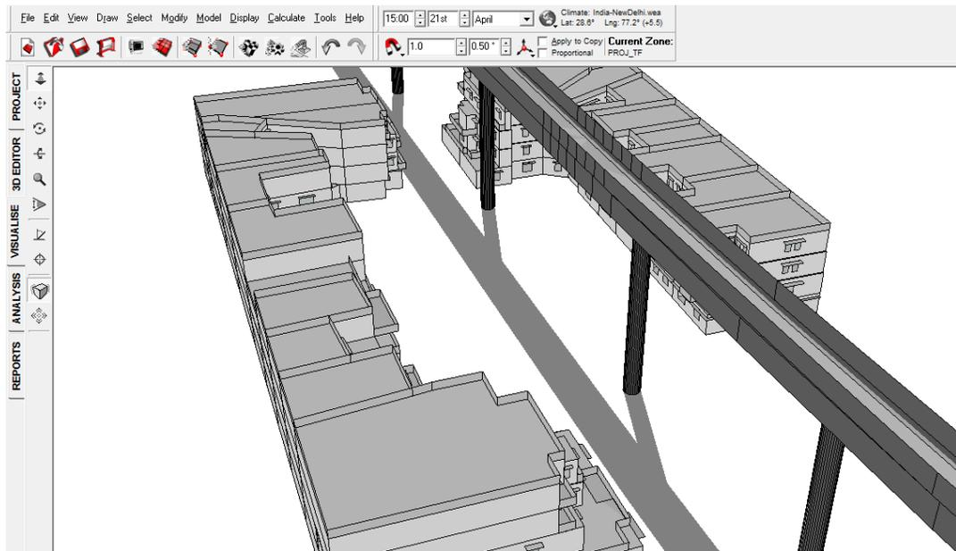
FIGURE 134: SHADOW RANGE ON 21<sup>ST</sup> APRIL 3 PM WITH VIADUCT
