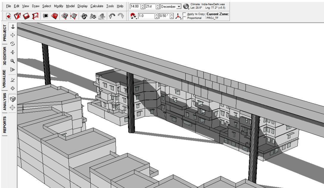
FIGURE 126: SHADOW RANGE ON 21<sup>ST</sup> DECEMBER 2 PM WITH VIADUCT
