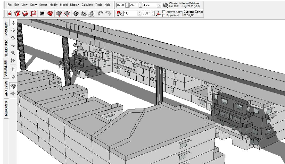
FIGURE 162: SHADOW RANGE ON 21<sup>ST</sup> JUNE 4 PM WITH VIADUCT
