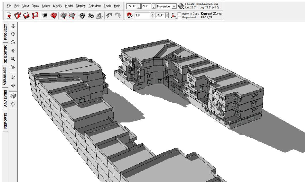
FIGURE 147: SHADOW RANGE ON 21<sup>ST</sup> NOVEMBER 3 PM WITHOUT VIADUCT
