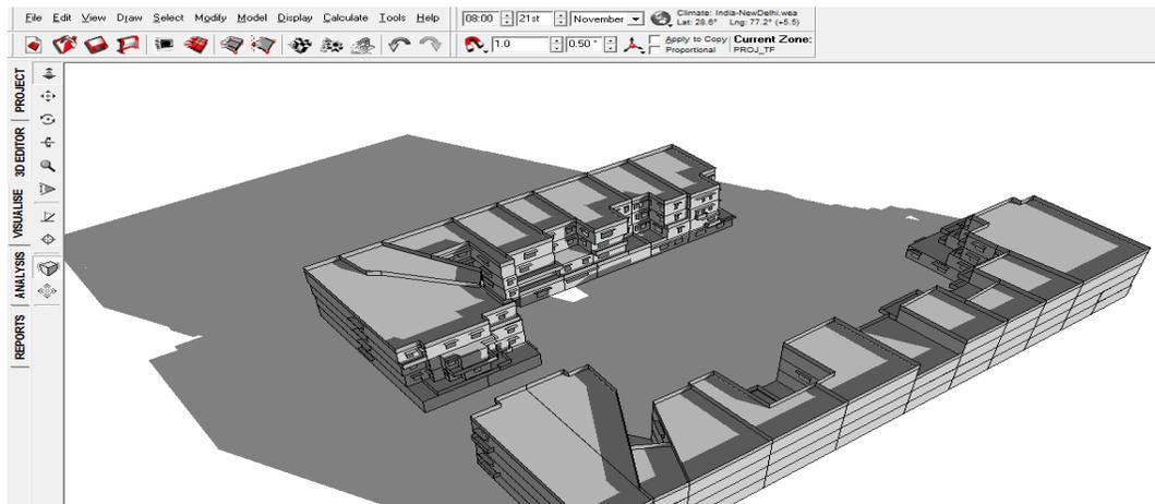
FIGURE 7: SHADOW RANGE ON 21<sup>ST</sup> NOVEMBER 8 AM WITHOUT VIADUCT
