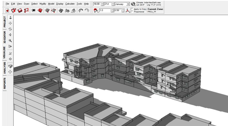
FIGURE 151: SHADOW RANGE ON 21<sup>ST</sup> JANUARY 4 PM WITHOUT VIADUCT
