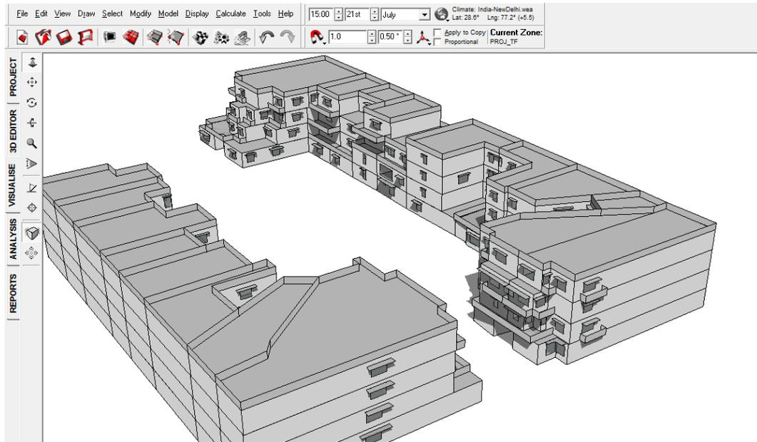
FIGURE 139: SHADOW RANGE ON 21<sup>ST</sup> JULY 3 PM WITHOUT VIADUCT
