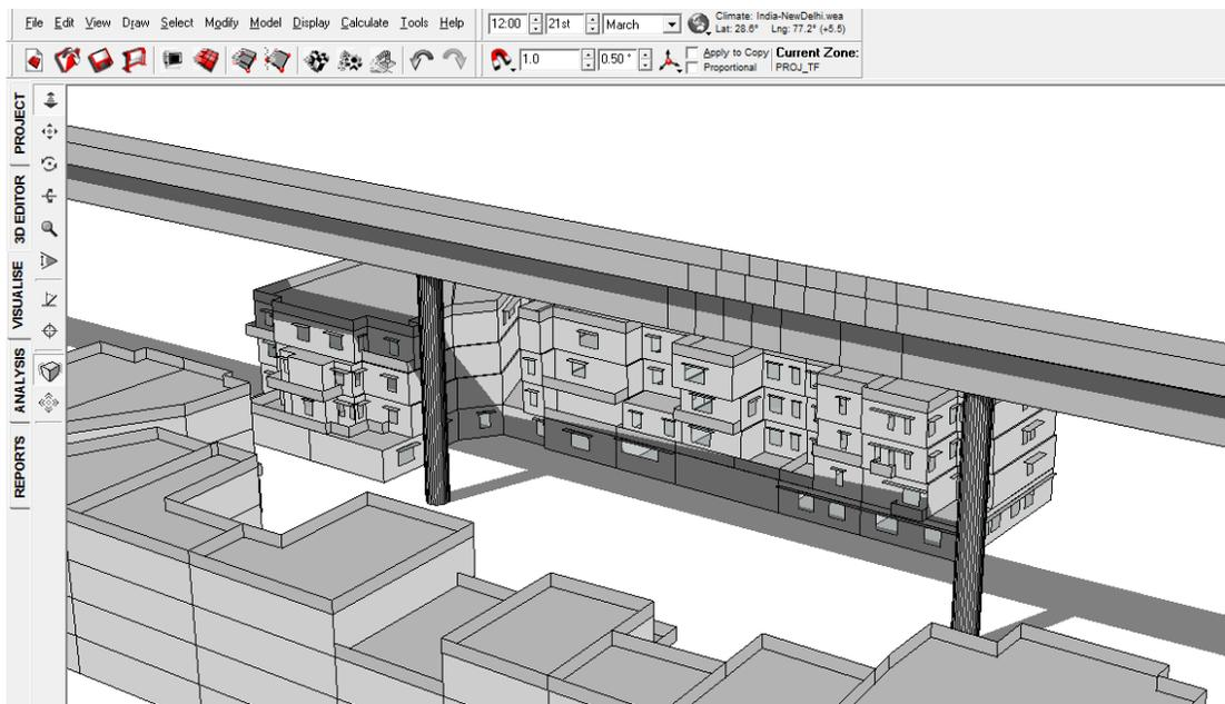
FIGURE 60: SHADOW RANGE ON 21<sup>ST</sup> MARCH 12 PM WITH VIADUCT
