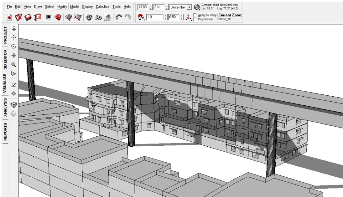
FIGURE 102: SHADOW RANGE ON 21<sup>ST</sup> DECEMBER 1 PM WITH VIADUCT
