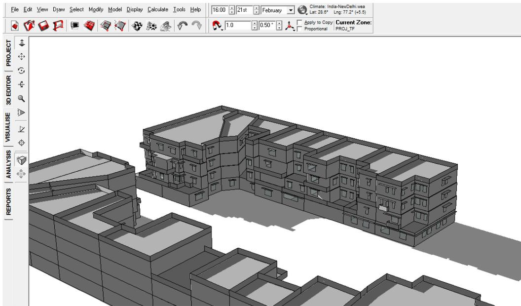
FIGURE 153: SHADOW RANGE ON 21<sup>ST</sup> FEBRUARY 4 PM WITHOUT VIADUCT
