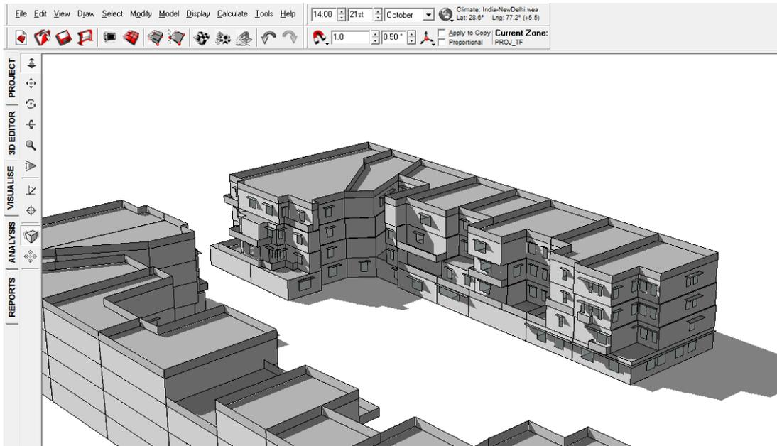
FIGURE 121: SHADOW RANGE ON 21<sup>ST</sup> OCTOBER 2 PM WITHOUT VIADUCT
