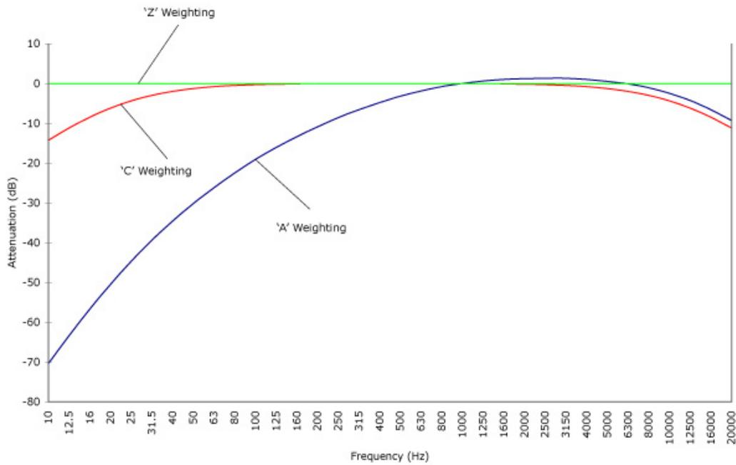
Fig. 2.3: Frequency Weighting Curves - 'A', 'C' & 'Z'
