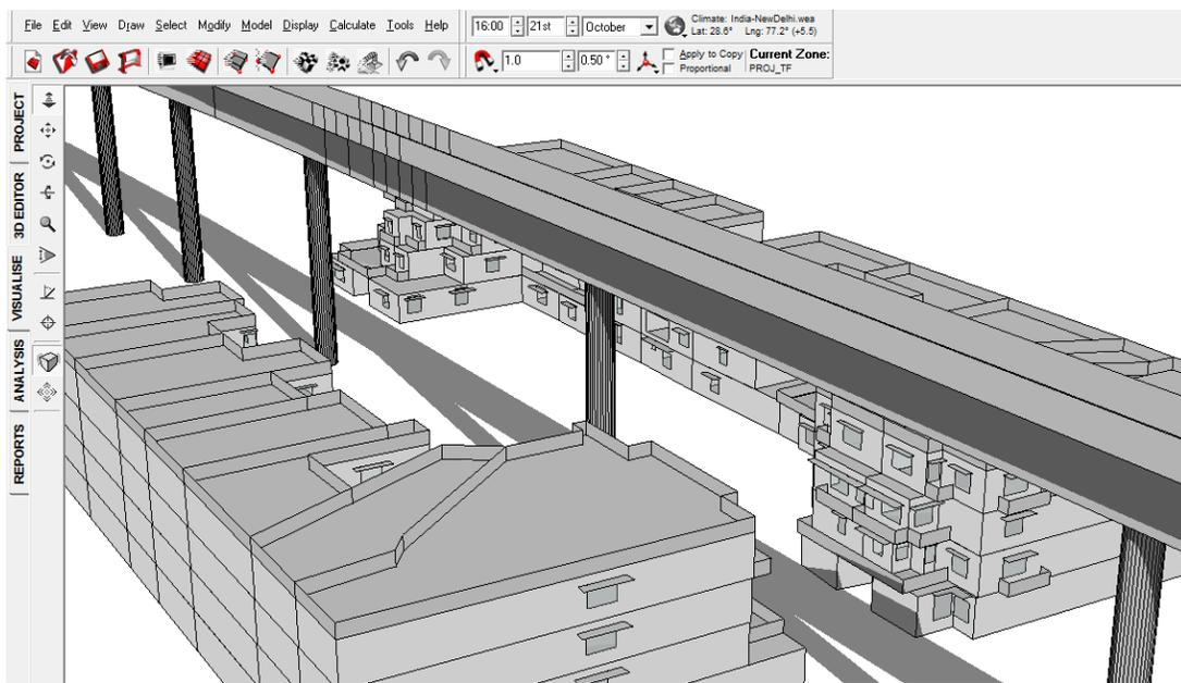
FIGURE 170: SHADOW RANGE ON 21<sup>ST</sup> OCTOBER 4 PM WITH VIADUCT
