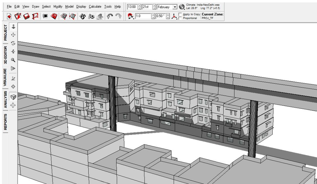
FIGURE 82: SHADOW RANGE ON 21<sup>ST</sup> FEBRUARY 1 PM WITH VIADUCT
