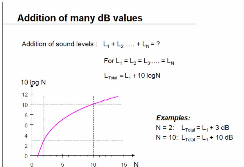
Fig. 2.4c: Addition of infinite sound pressure levels
