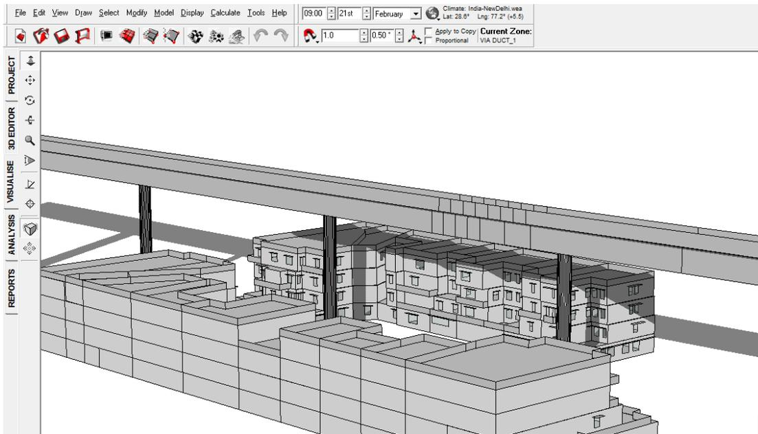
FIGURE 22: SHADOW RANGE ON 21<sup>ST</sup> FEBRUARY 9 AM WITH VIADUCT
