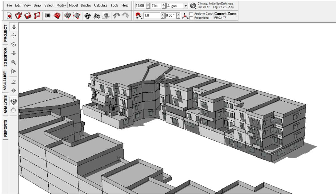
FIGURE 93: SHADOW RANGE ON 21<sup>ST</sup> AUGUST 1 PM WITHOUT VIADUCT
