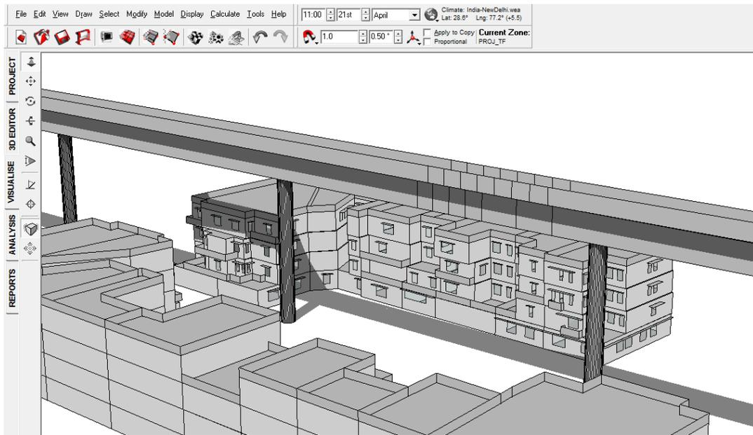
FIGURE 38: SHADOW RANGE ON 21<sup>ST</sup> APRIL 11 AM WITH VIADUCT
