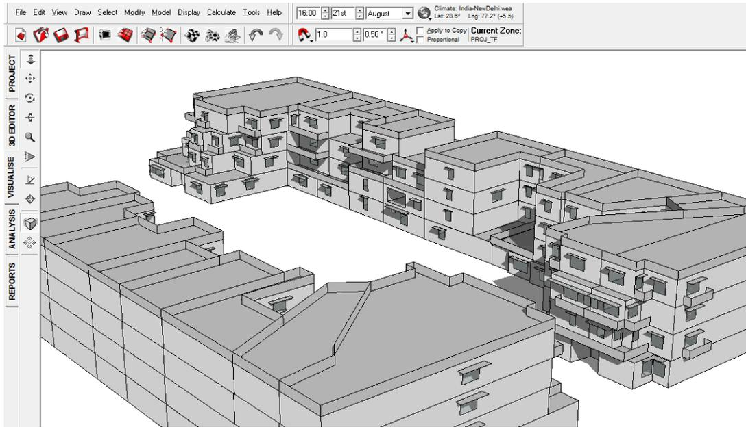
FIGURE 165: SHADOW RANGE ON 21<sup>ST</sup> AUGUST 4 PM WITHOUT VIADUCT
