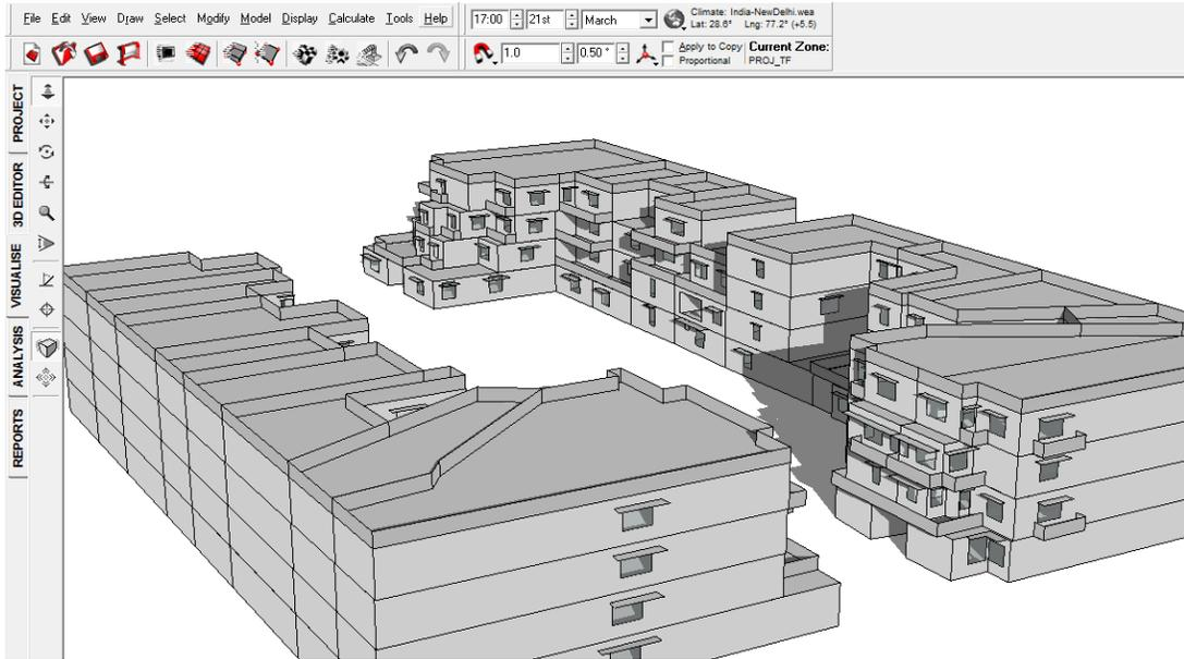
FIGURE 179: SHADOW RANGE ON 21<sup>ST</sup> MARCH 5 PM WITHOUT VIADUCT
