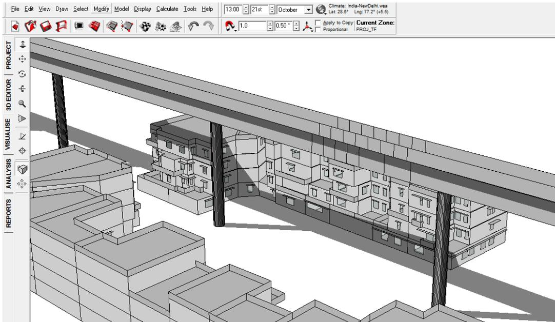
FIGURE 98: SHADOW RANGE ON 21<sup>ST</sup> OCTOBER 1 PM WITH VIADUCT
