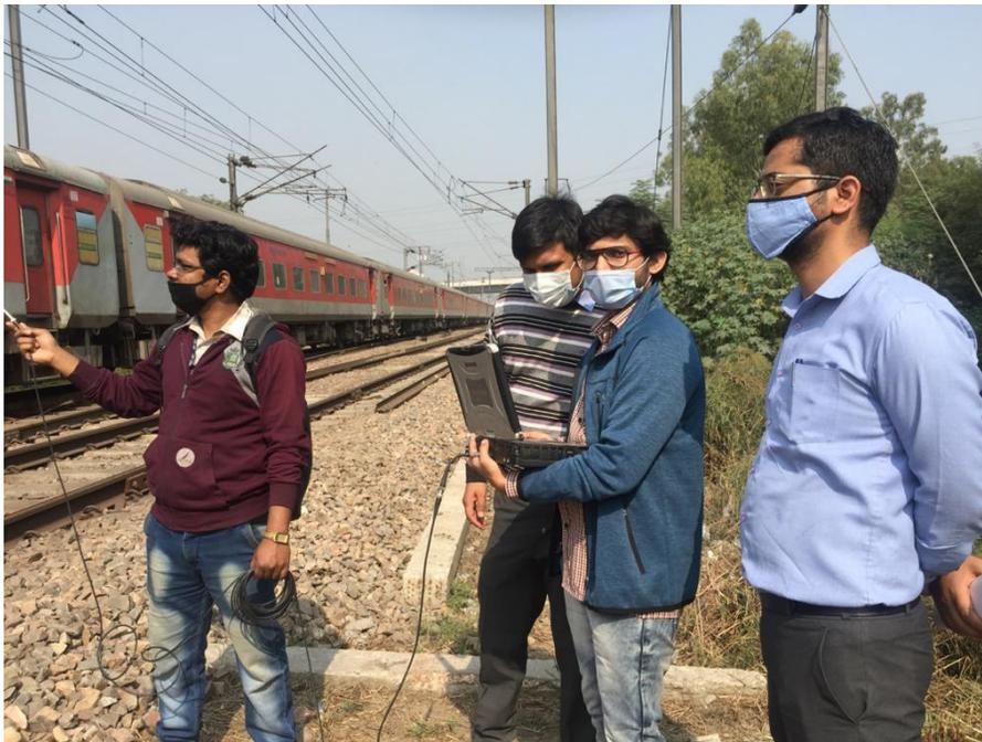
Photo 3.6 Noise Monitoring at Railway Track
