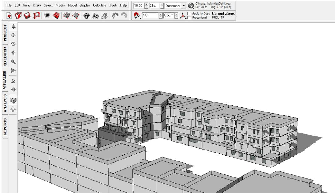
FIGURE 25: SHADOW RANGE ON 21<sup>ST</sup> DECEMBER 10 AM WITHOUT VIADUCT
