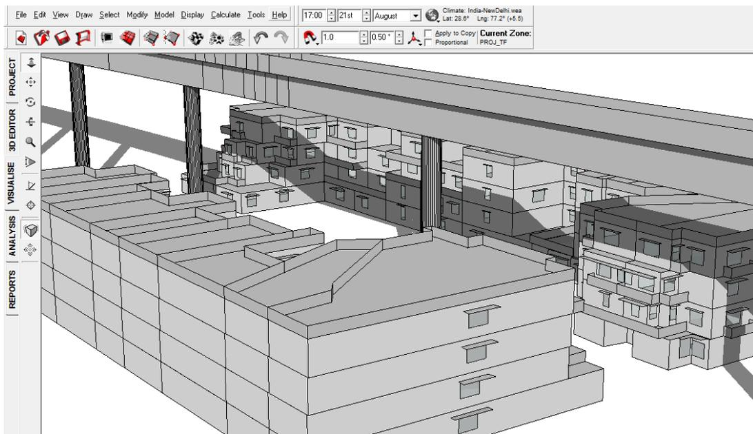
FIGURE 190: SHADOW RANGE ON 21<sup>ST</sup> AUGUST 5 PM WITH VIADUCT
