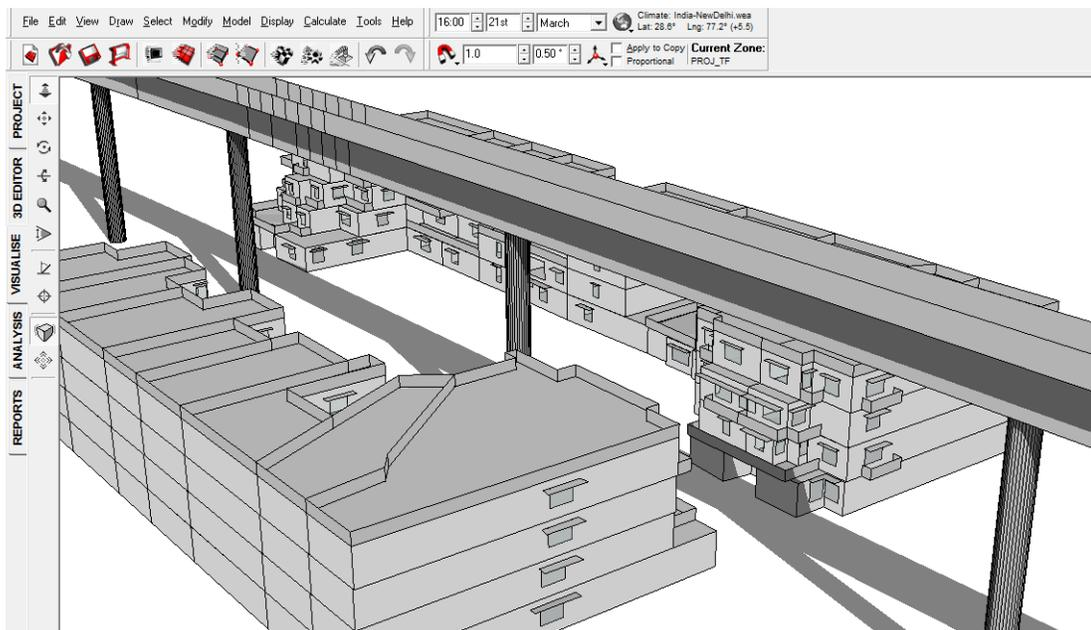
FIGURE 156: SHADOW RANGE ON 21<sup>ST</sup> MARCH 4 PM WITH VIADUCT
