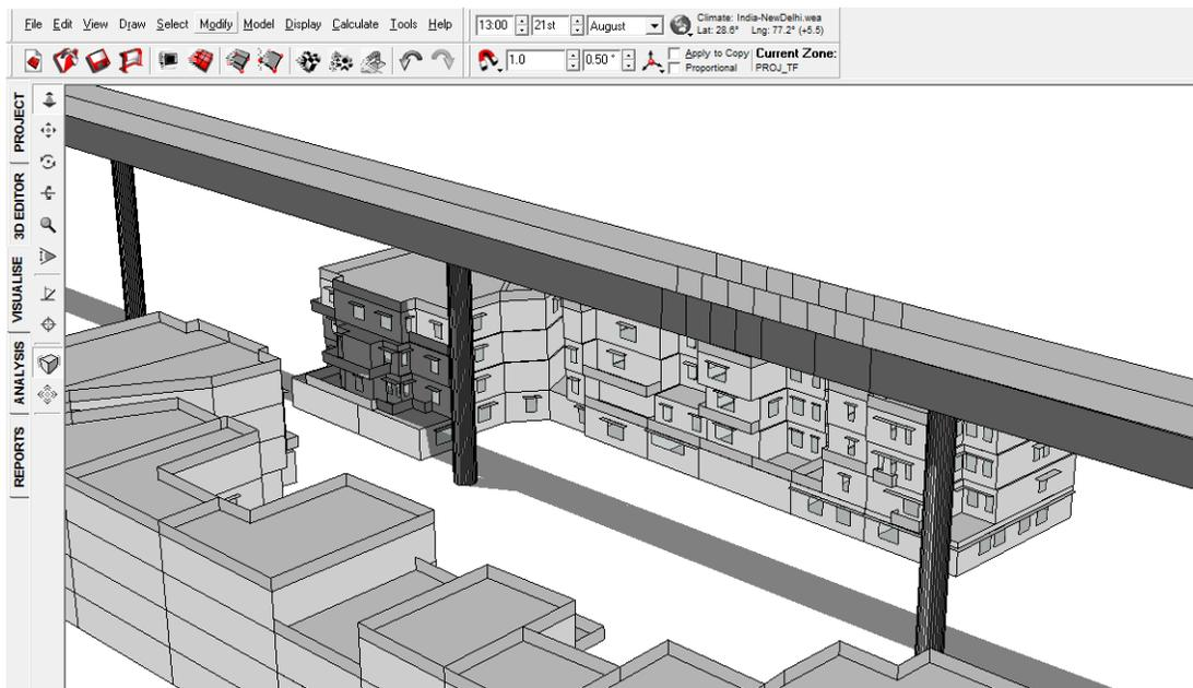
FIGURE 94: SHADOW RANGE ON 21<sup>ST</sup> AUGUST 1 PM WITH VIADUCT
