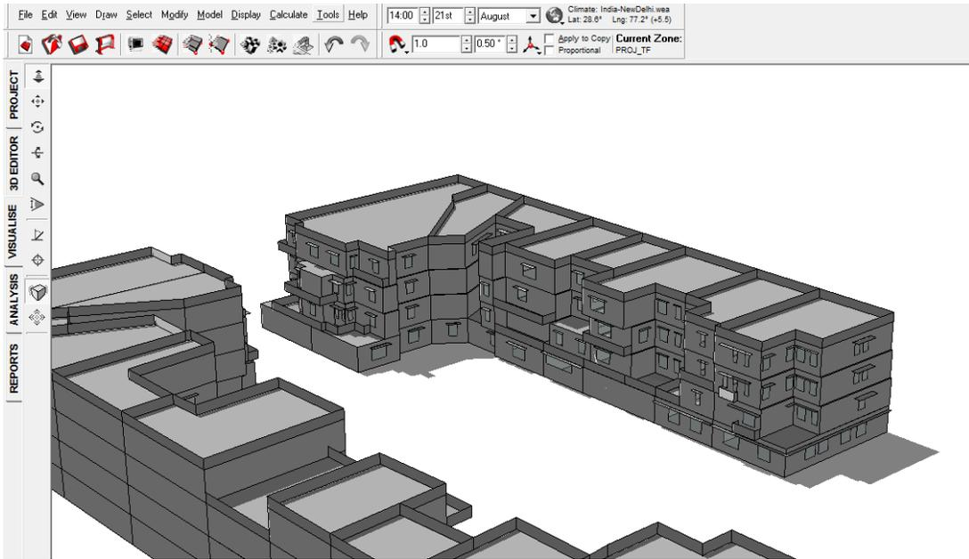
FIGURE 117: SHADOW RANGE ON 21<sup>ST</sup> AUGUST 2 PM WITHOUT VIADUCT
