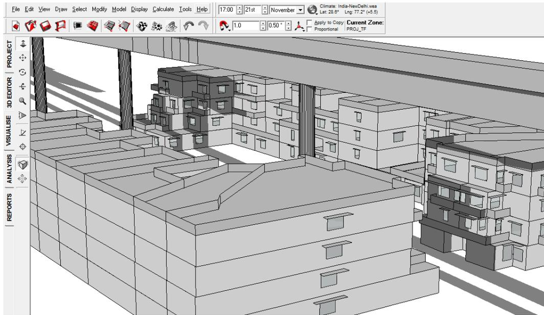
FIGURE 196: SHADOW RANGE ON 21<sup>ST</sup> NOVEMBER 5 PM WITH VIADUCT
