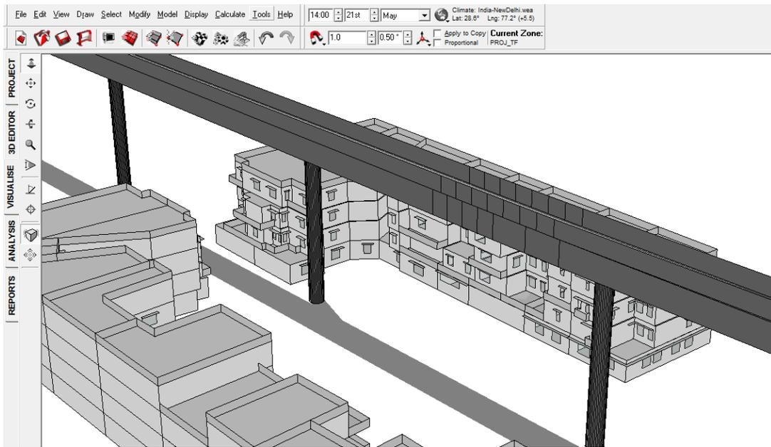
FIGURE 112: SHADOW RANGE ON 21<sup>ST</sup> MAY 2 PM WITH VIADUCT
