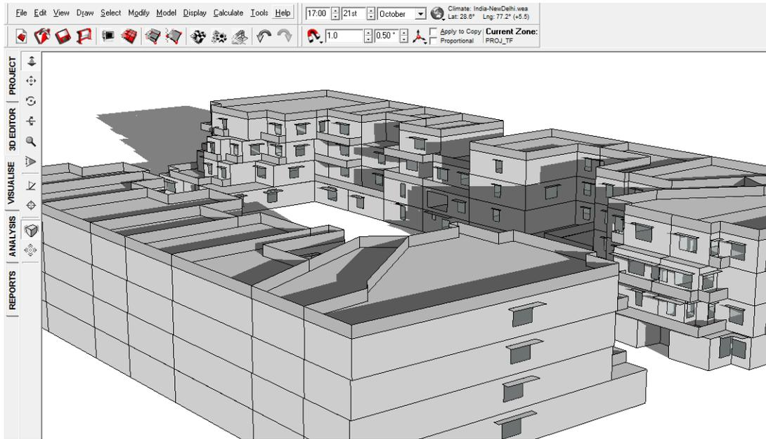
FIGURE 193: SHADOW RANGE ON 21<sup>ST</sup> OCTOBER 5 PM WITHOUT VIADUCT
