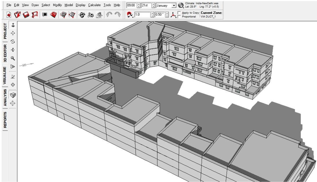
FIGURE 19: SHADOW RANGE ON 21<sup>ST</sup> JANUARY 9 AM WITHOUT VIADUCT
