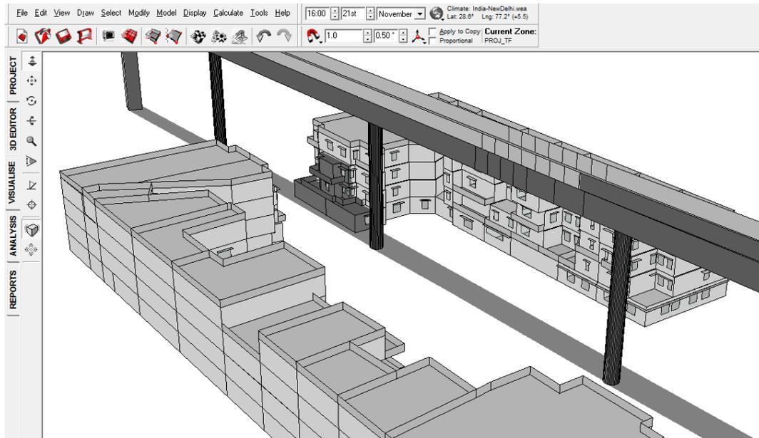
FIGURE 172: SHADOW RANGE ON 21<sup>ST</sup> NOVEMBER 4 PM WITH VIADUCT
