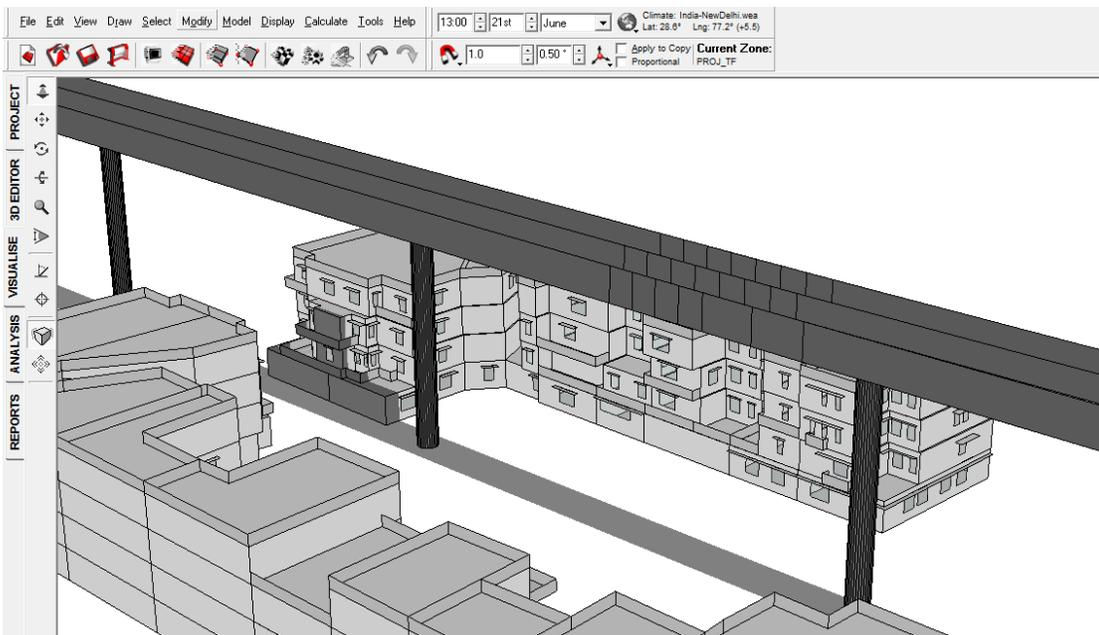
FIGURE 90: SHADOW RANGE ON 21<sup>ST</sup> JUNE 1 PM WITH VIADUCT
