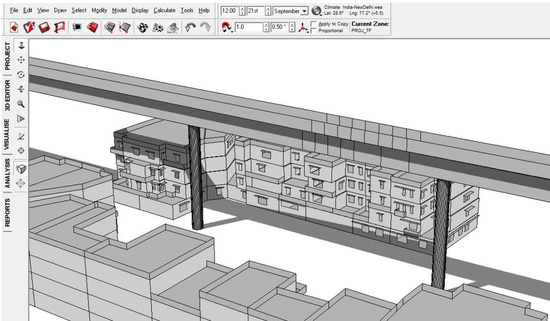
FIGURE 72: SHADOW RANGE ON 21<sup>ST</sup> SEPTEMBER 12 PM WITH VIADUCT
