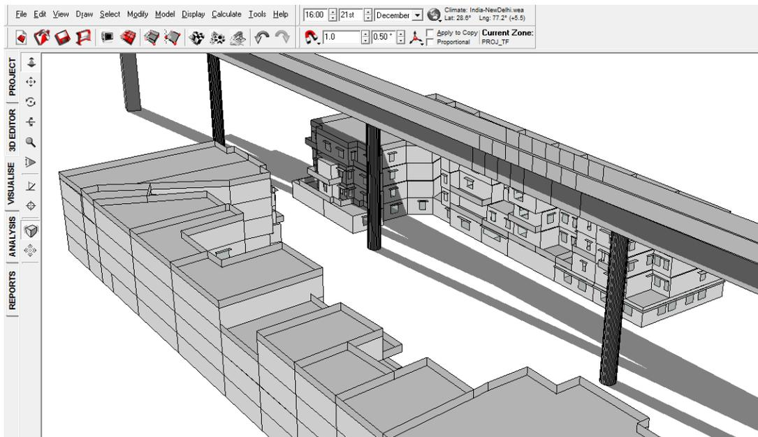
FIGURE 174: SHADOW RANGE ON 21<sup>ST</sup> DECEMBER 4 PM WITH VIADUCT
