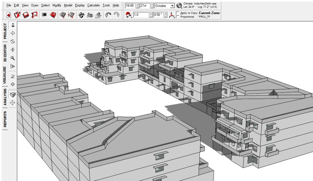
FIGURE 169: SHADOW RANGE ON 21<sup>ST</sup> OCTOBER 4 PM WITHOUT VIADUCT
