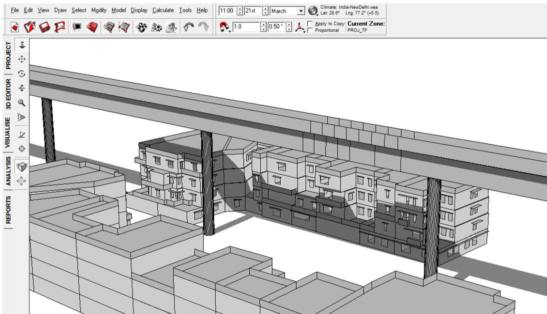
FIGURE 36: SHADOW RANGE ON 21<sup>ST</sup> MARCH 11 AM WITH VIADUCT
