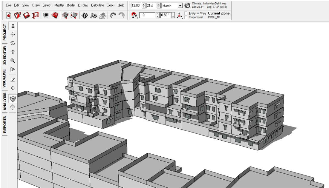
FIGURE 59: SHADOW RANGE ON 21<sup>ST</sup> MARCH 12 PM WITHOUT VIADUCT
