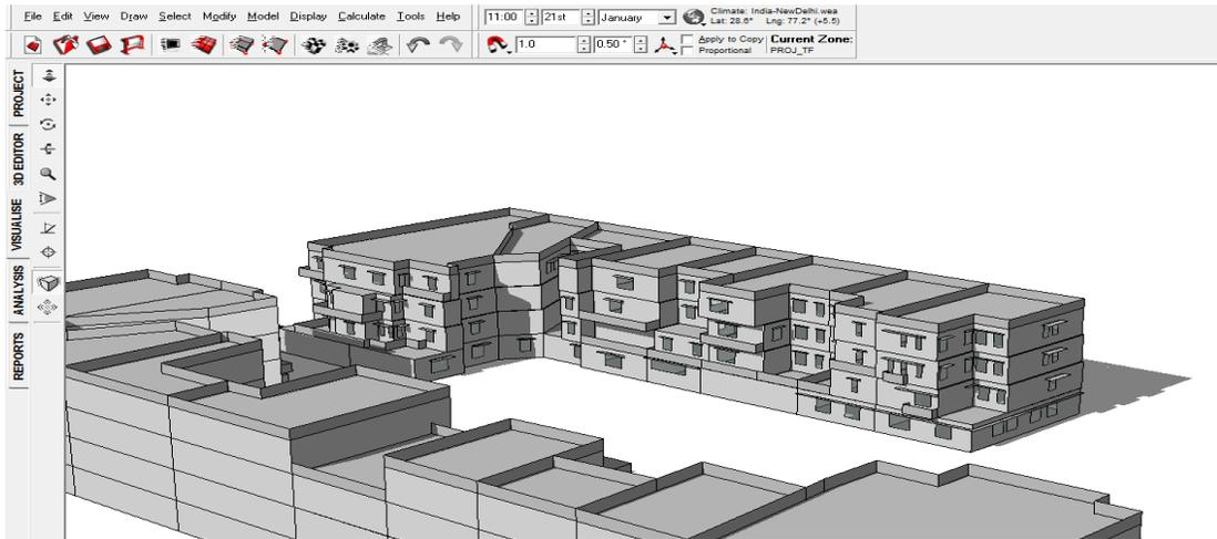
FIGURE 31: SHADOW RANGE ON 21<sup>ST</sup> JANUARY 11 AM WITHOUT VIADUCT
