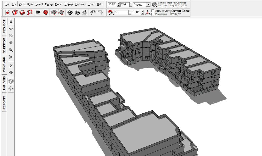
FIGURE 141: SHADOW RANGE ON 21<sup>ST</sup> AUGUST 3 PM WITHOUT VIADUCT
