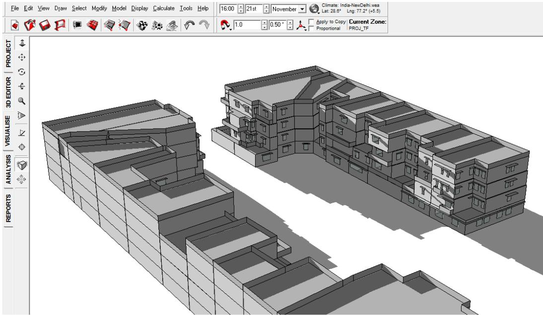
FIGURE 171: SHADOW RANGE ON 21<sup>ST</sup> NOVEMBER 4 PM WITHOUT VIADUCT
