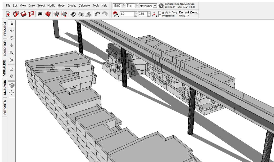
FIGURE 148: SHADOW RANGE ON 21<sup>ST</sup> NOVEMBER 3 PM WITH VIADUCT
