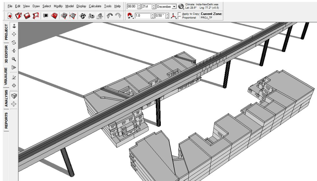
FIGURE 10: SHADOW RANGE ON 21<sup>ST</sup> DECEMBER 8 AM WITH VIADUCT
