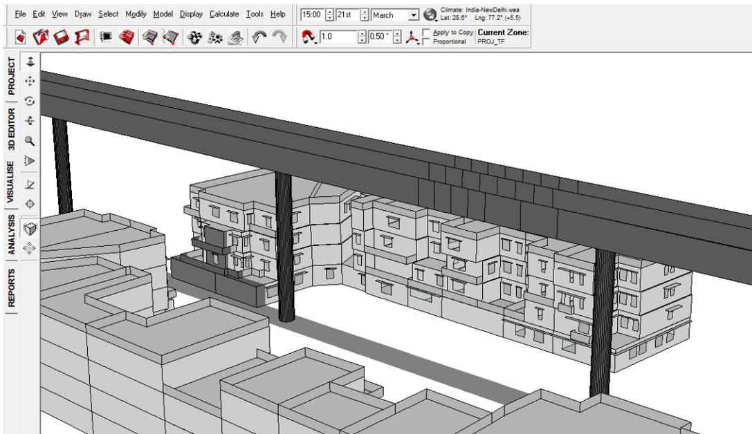
FIGURE 132: SHADOW RANGE ON 21<sup>ST</sup> MARCH 3 PM WITH VIADUCT
