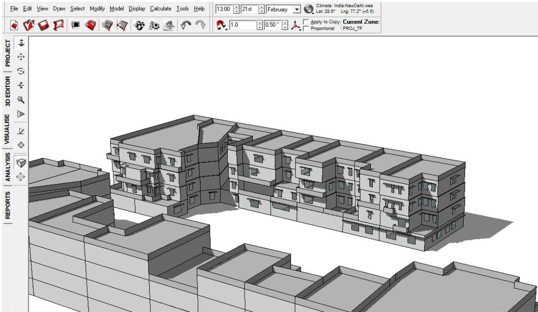
FIGURE 81: SHADOW RANGE ON 21<sup>ST</sup> FEBRUARY 1 PM WITHOUT VIADUCT
