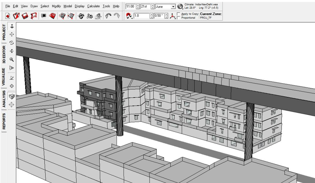
FIGURE 42: SHADOW RANGE ON 21<sup>ST</sup> JUNE 11 AM WITH VIADUCT
