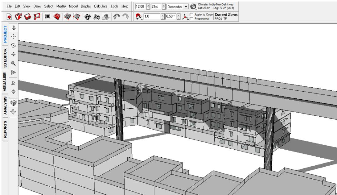
FIGURE 78: SHADOW RANGE ON 21<sup>ST</sup> DECEMBER 12 PM WITH VIADUCT
