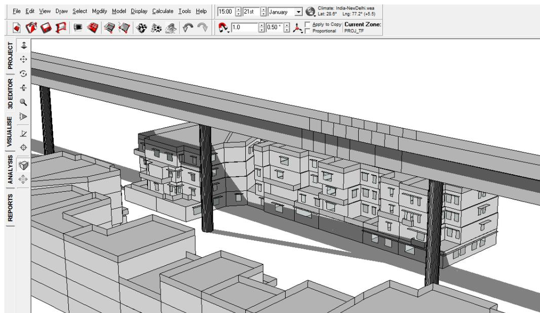
FIGURE 128: SHADOW RANGE ON 21<sup>ST</sup> JANUARY 3 PM WITH VIADUCT
