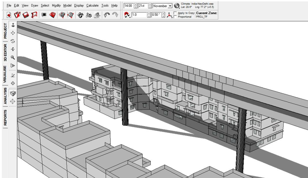
FIGURE 124: SHADOW RANGE ON 21<sup>ST</sup> NOVEMBER 2 PM WITH VIADUCT
