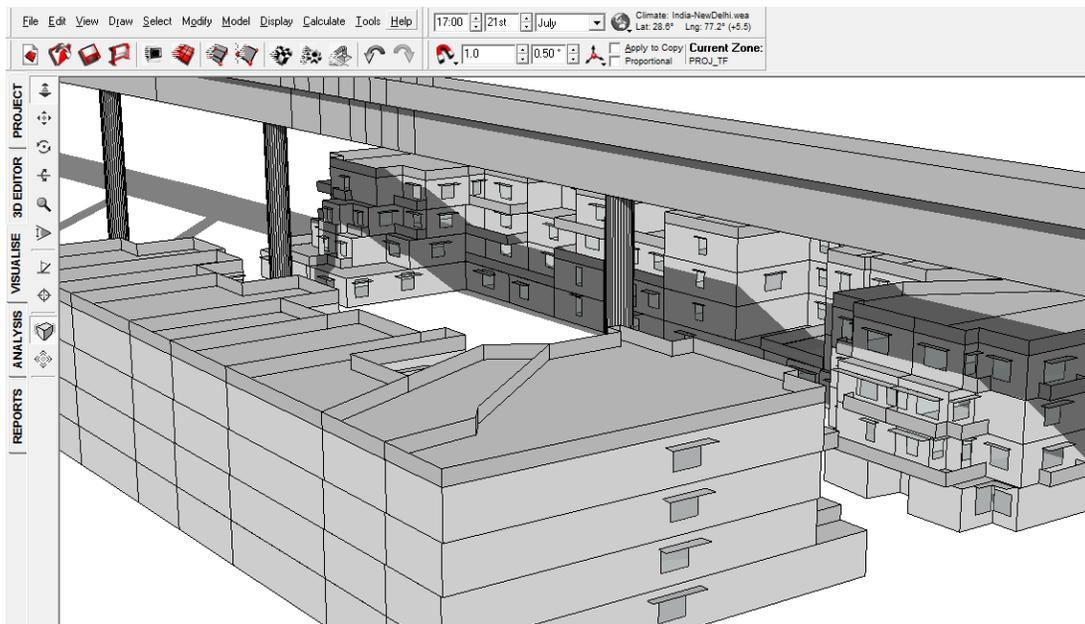
FIGURE 188: SHADOW RANGE ON 21<sup>ST</sup> JULY 5 PM WITH VIADUCT
