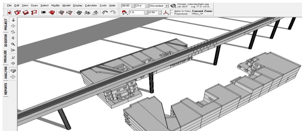
FIGURE 8: SHADOW RANGE ON 21<sup>ST</sup> NOVEMBER 8 AM WITH VIADUCT
