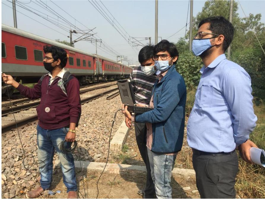
Photo 3.7 Noise Monitoring at Railway Track
