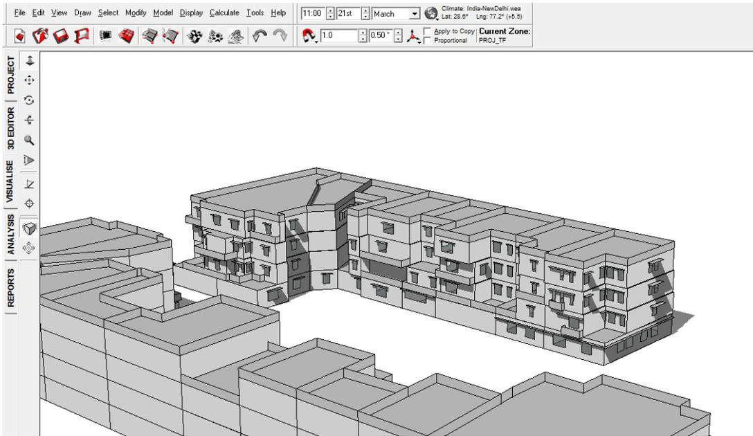
FIGURE 35: SHADOW RANGE ON 21<sup>ST</sup> MARCH 11 AM WITHOUT VIADUCT
