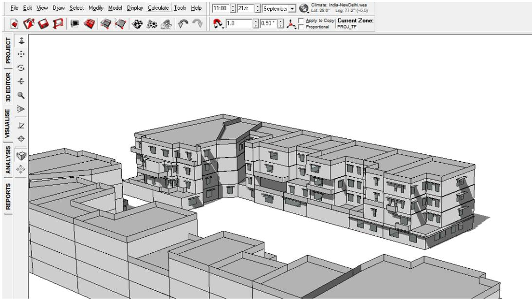
FIGURE 47: SHADOW RANGE ON 21<sup>ST</sup> SEPTEMBER 11 AM WITHOUT VIADUCT
