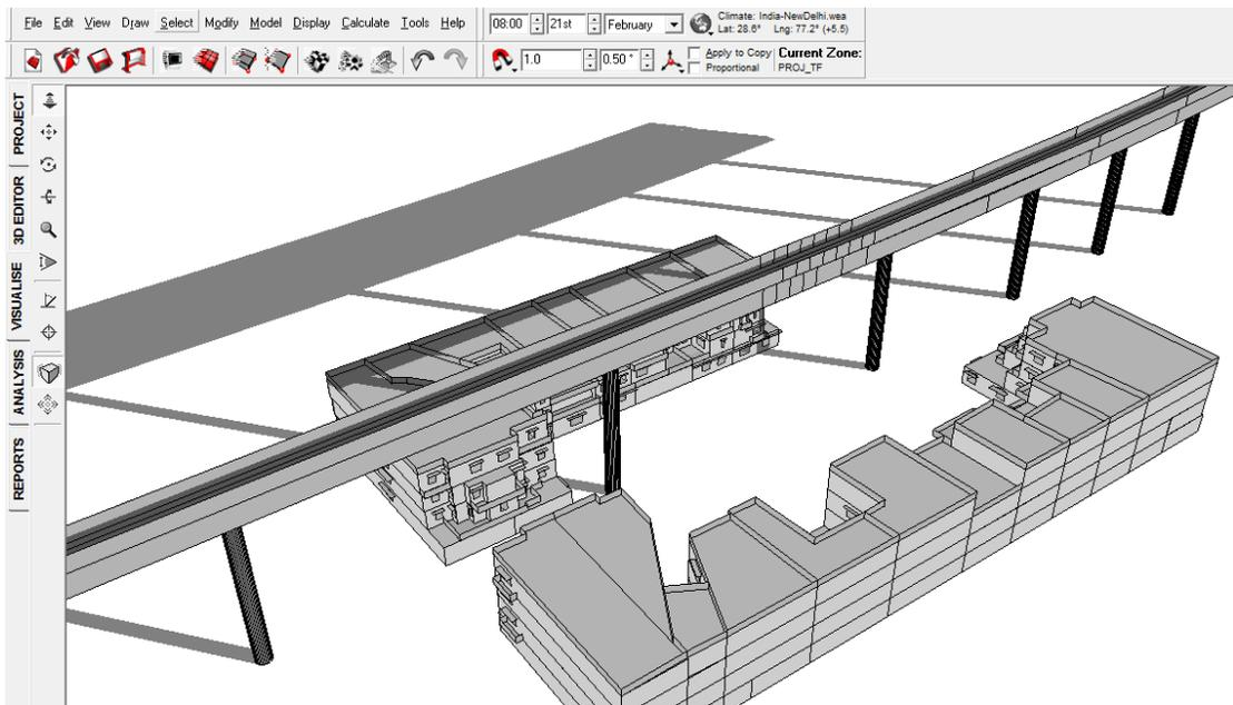
FIGURE 14: SHADOW RANGE ON 21<sup>ST</sup> FEBRUARY 8 AM WITH VIADUCT
