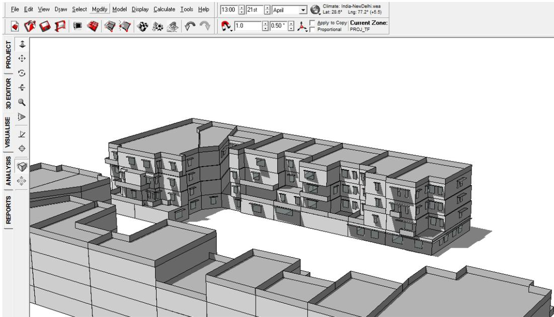
FIGURE 85: SHADOW RANGE ON 21<sup>ST</sup> APRIL 1 PM WITHOUT VIADUCT
