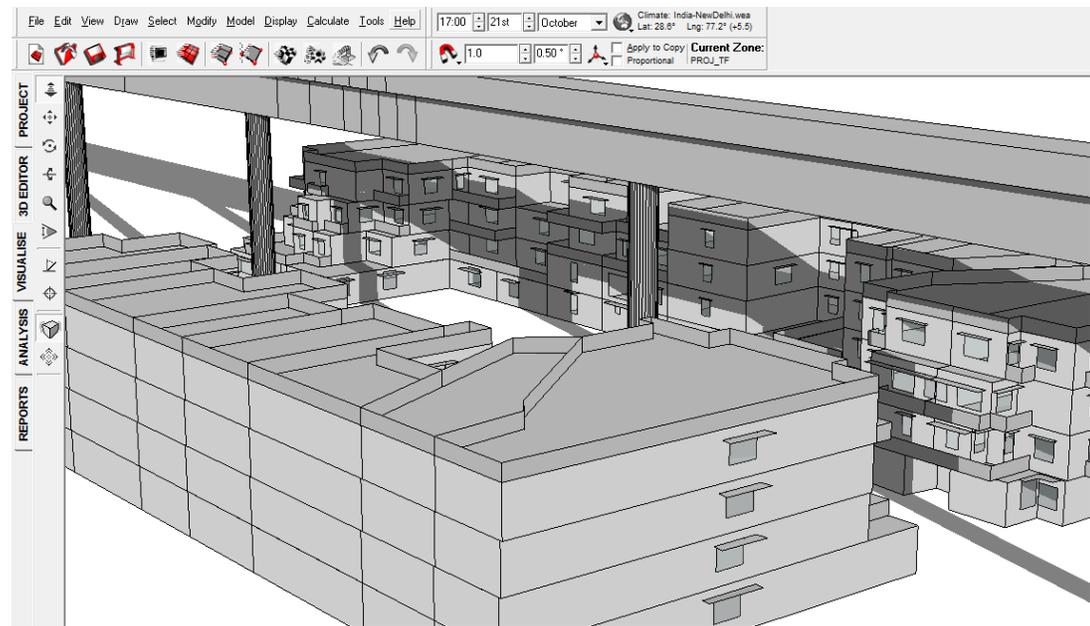
FIGURE 194: SHADOW RANGE ON 21<sup>ST</sup> OCTOBER 5 PM WITH VIADUCT
