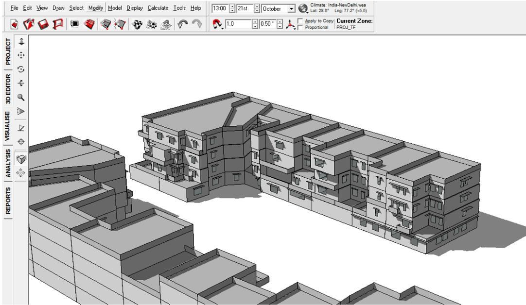
FIGURE 97: SHADOW RANGE ON 21<sup>ST</sup> OCTOBER 1 PM WITHOUT VIADUCT
