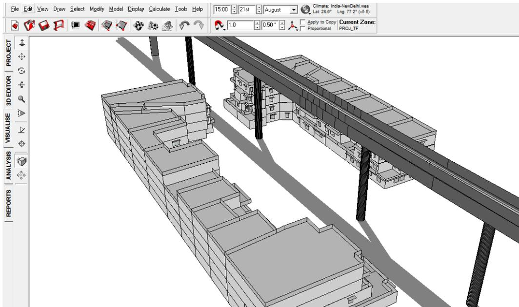
FIGURE 142: SHADOW RANGE ON 21<sup>ST</sup> AUGUST 3 PM WITH VIADUCT
