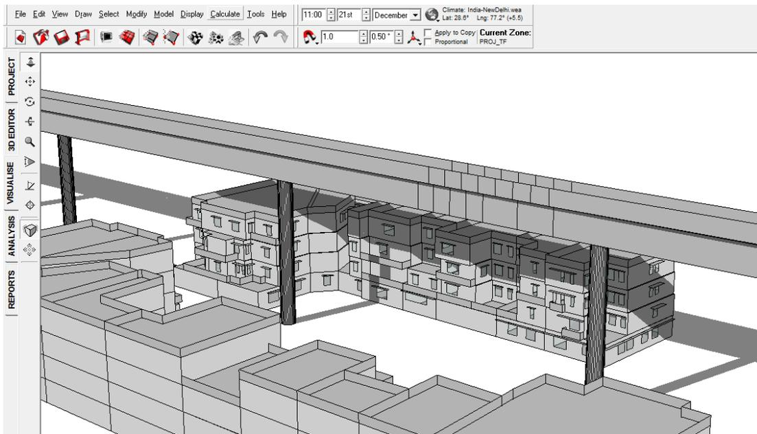
FIGURE 54: SHADOW RANGE ON 21<sup>ST</sup> DECEMBER 11 AM WITH VIADUCT
