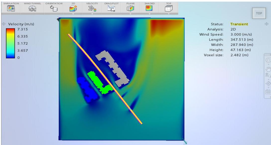
FIGURE 205: WIND ANALYSIS RESULT – WITH VIADUCT
