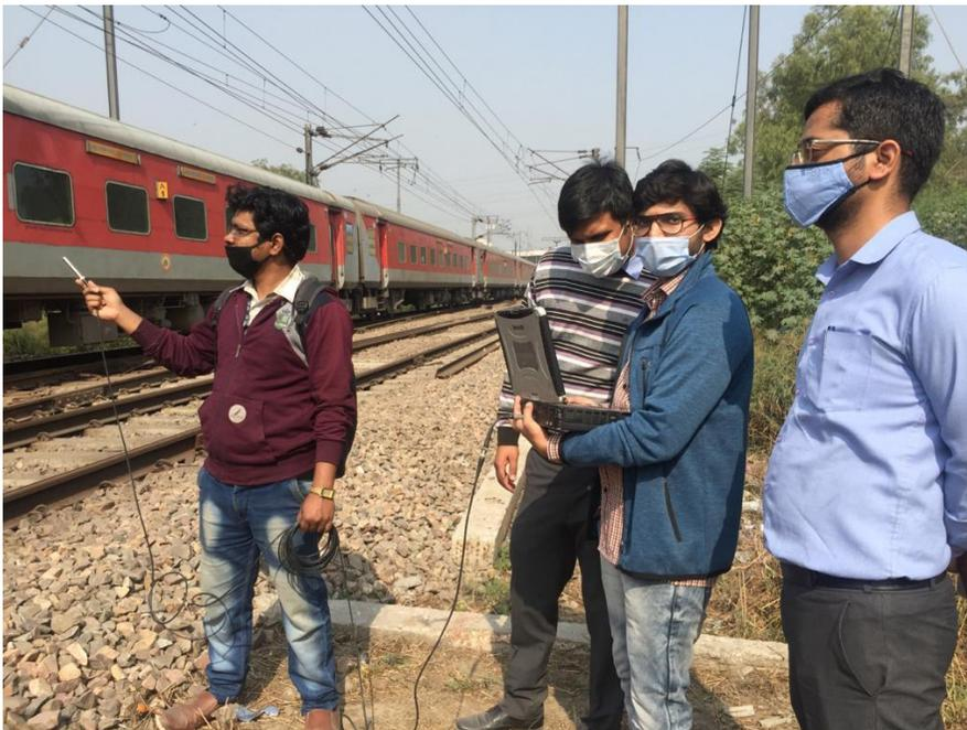
Photo 3.3 Noise Monitoring at Railway Track
