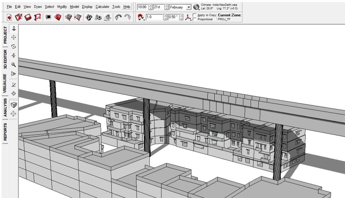
FIGURE 30: SHADOW RANGE ON 21<sup>ST</sup> FEBRUARY 10 AM WITH VIADUCT
