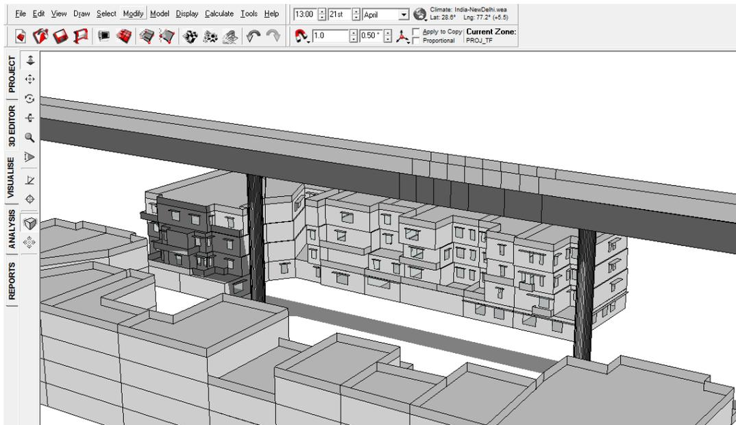
FIGURE 86: SHADOW RANGE ON 21<sup>ST</sup> APRIL 1 PM WITH VIADUCT
