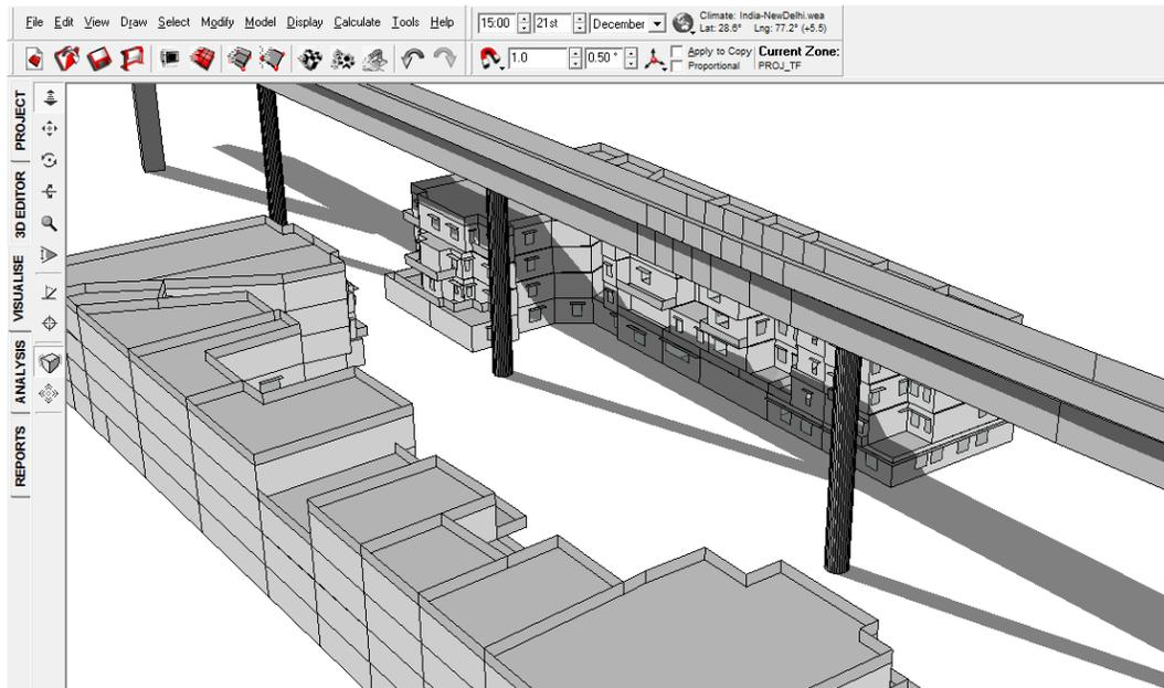
FIGURE 150: SHADOW RANGE ON 21<sup>ST</sup> DECEMBER 3 PM WITH VIADUCT
