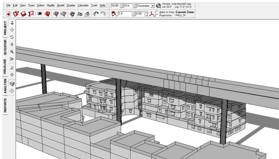
FIGURE 26: SHADOW RANGE ON 21<sup>ST</sup> DECEMBER 10 AM WITH VIADUCT
