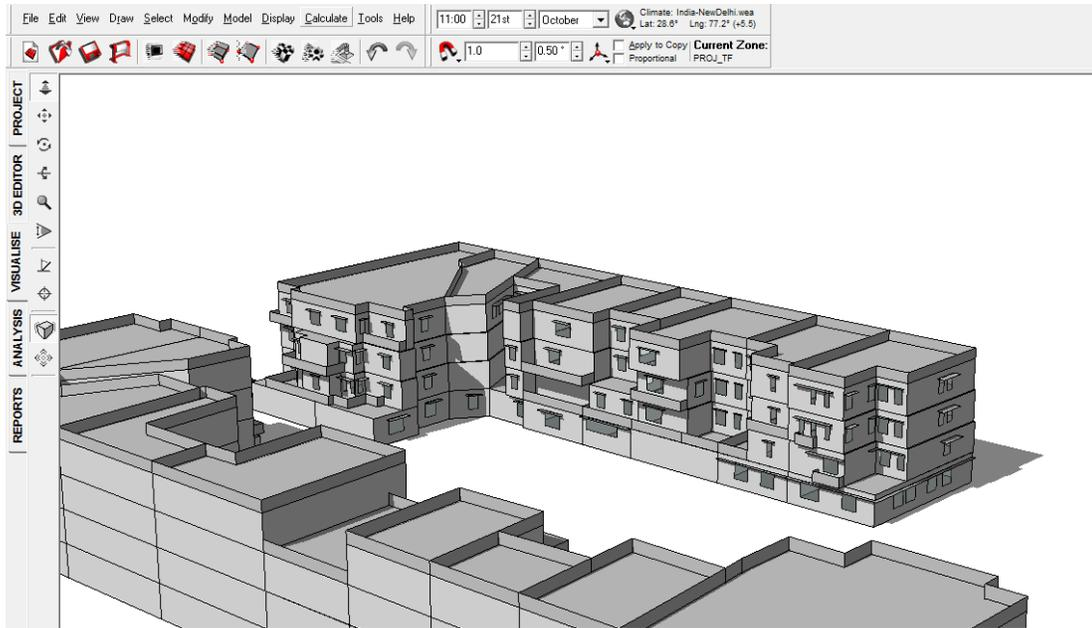
FIGURE 49: SHADOW RANGE ON 21<sup>ST</sup> OCTOBER 11 AM WITHOUT VIADUCT
