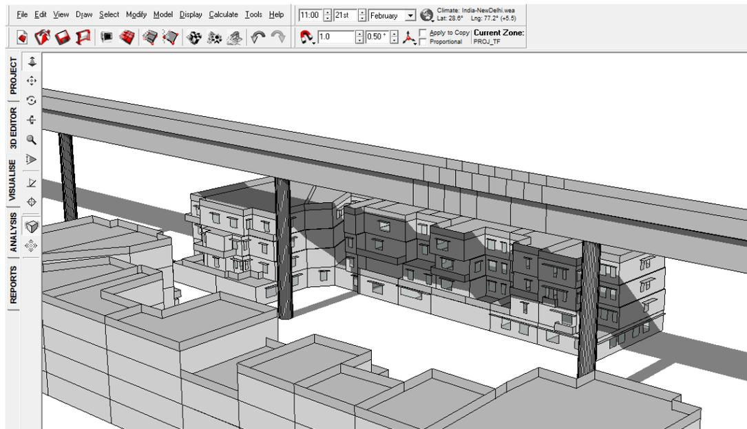
FIGURE 34: SHADOW RANGE ON 21<sup>ST</sup> FEBRUARY 11 AM WITH VIADUCT
