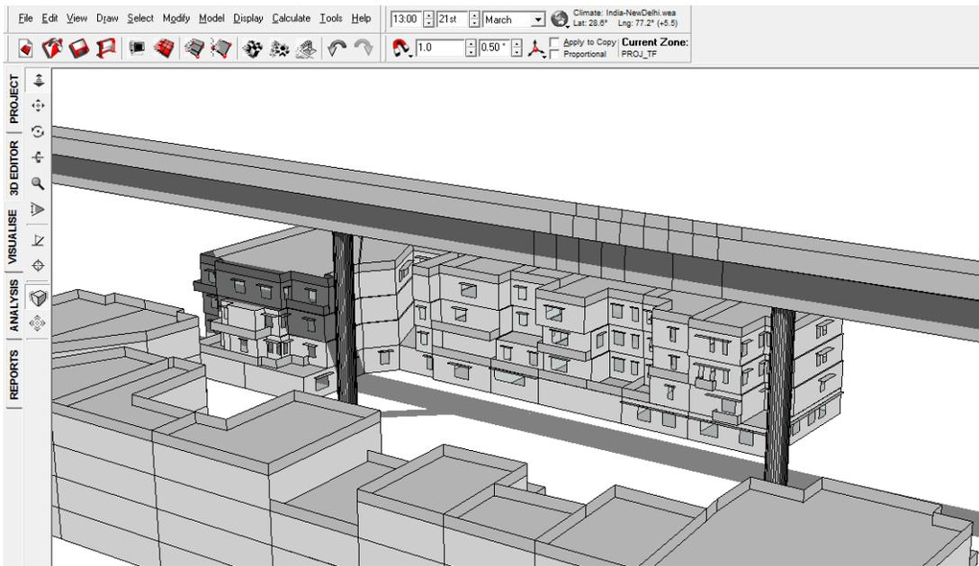
FIGURE 84: SHADOW RANGE ON 21<sup>ST</sup> MARCH 1 PM WITH VIADUCT
