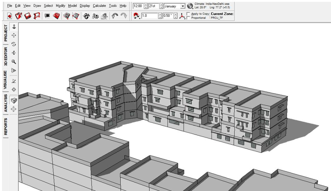
FIGURE 55: SHADOW RANGE ON 21<sup>ST</sup> JANUARY 12 PM WITHOUT VIADUCT
