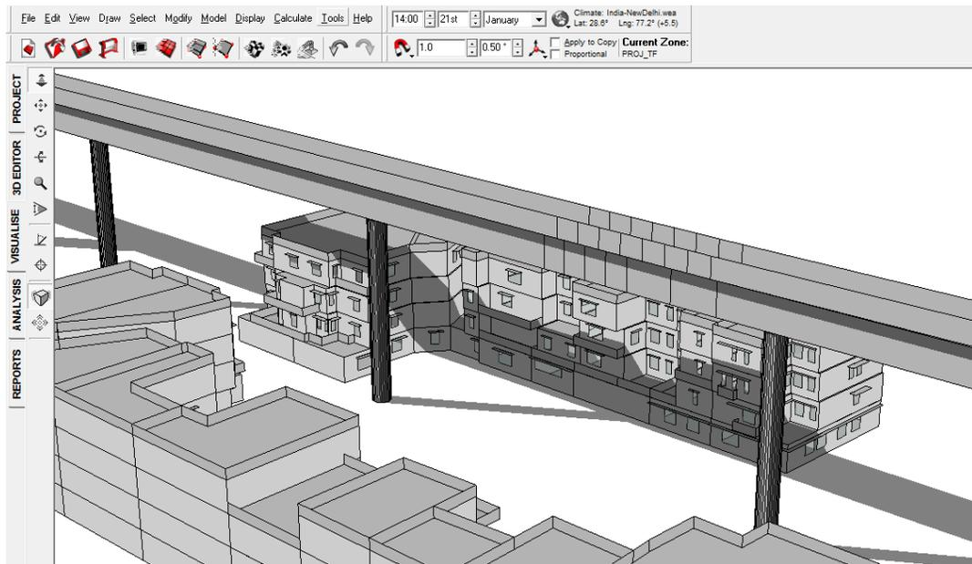
FIGURE 104: SHADOW RANGE ON 21<sup>ST</sup> JANUARY 2 PM WITH VIADUCT
