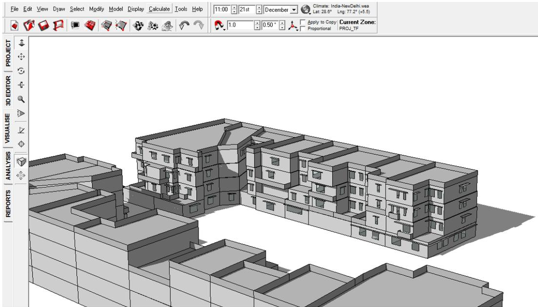
FIGURE 53: SHADOW RANGE ON 21<sup>ST</sup> DECEMBER 11 AM WITHOUT VIADUCT
