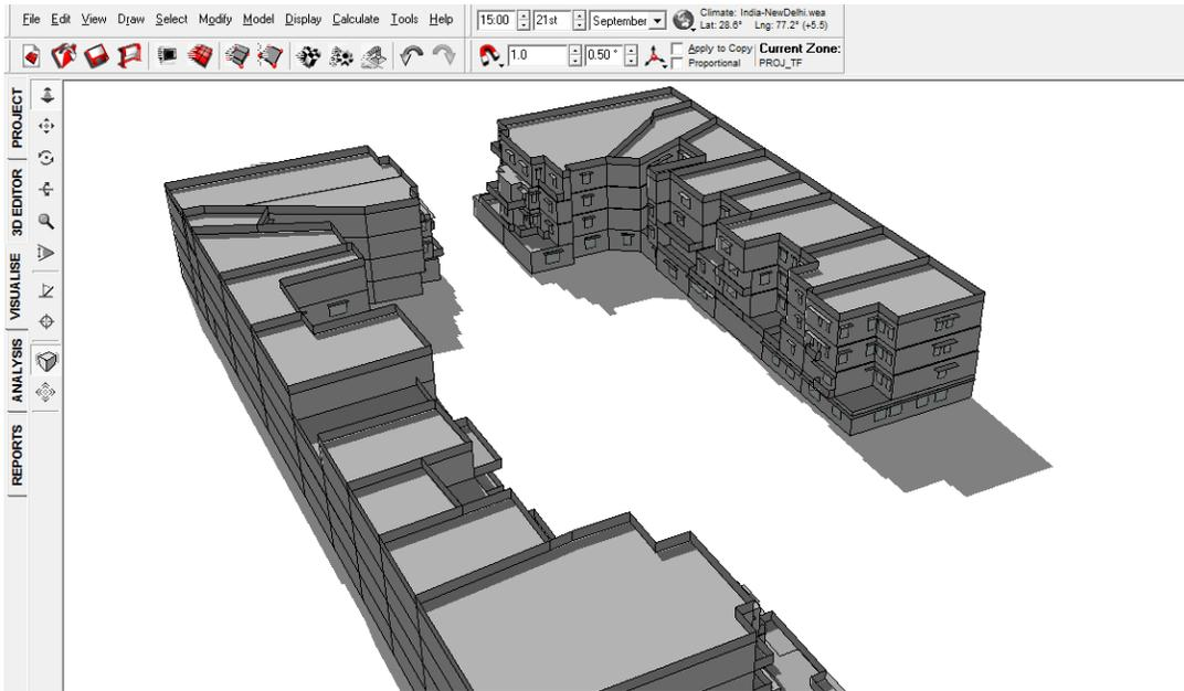
FIGURE 143: SHADOW RANGE ON 21<sup>ST</sup> SEPTEMBER 3 PM WITHOUT VIADUCT
