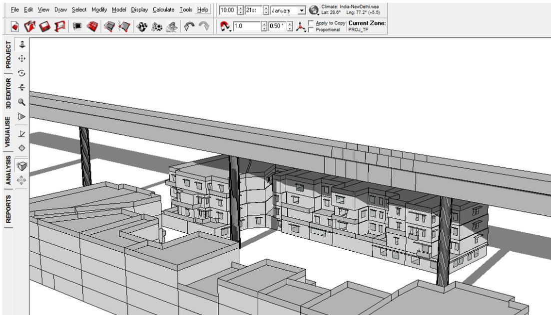
FIGURE 28: SHADOW RANGE ON 21<sup>ST</sup> JANUARY 10 AM WITH VIADUCT
