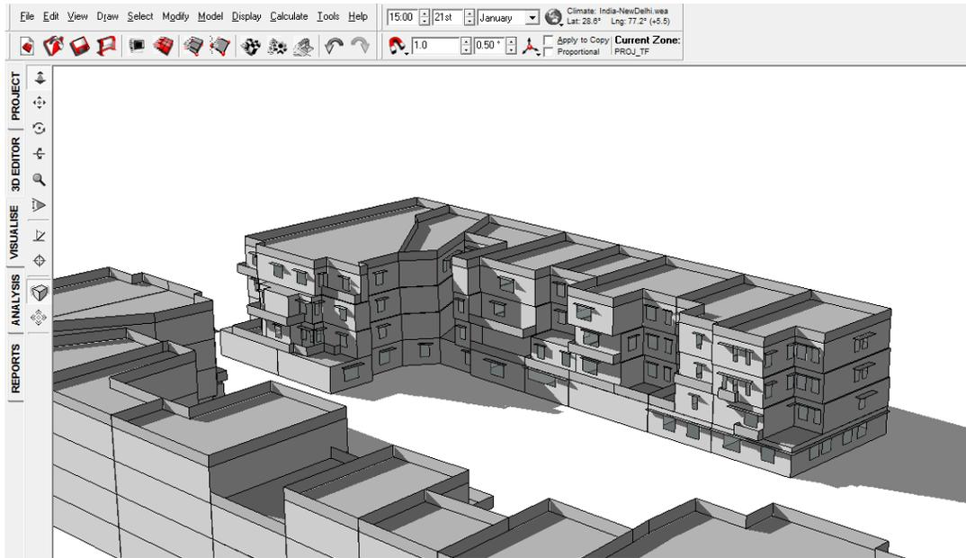
FIGURE 127: SHADOW RANGE ON 21<sup>ST</sup> JANUARY 3 PM WITHOUT VIADUCT
