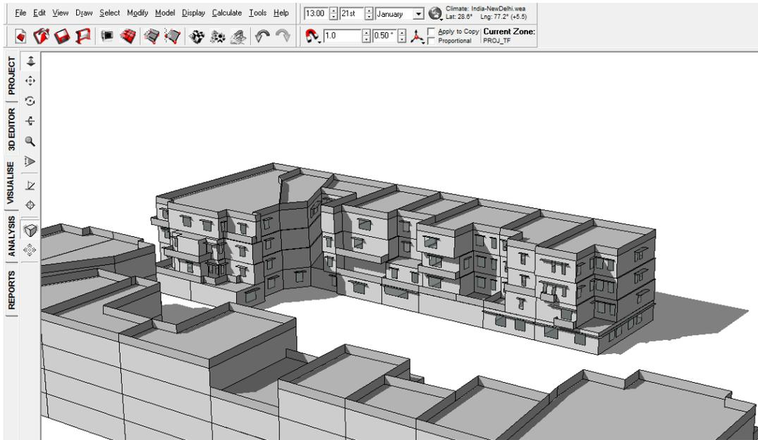
FIGURE 79: SHADOW RANGE ON 21<sup>ST</sup> JANUARY 1 PM WITHOUT VIADUCT
