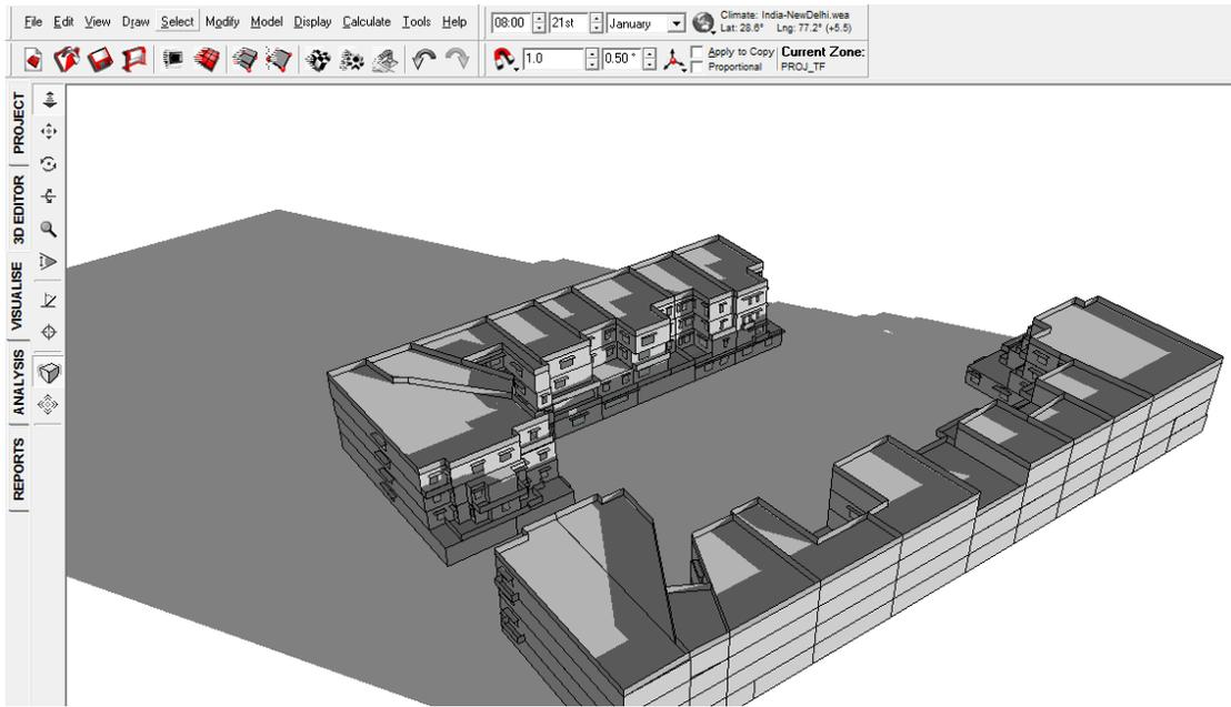
FIGURE 11: SHADOW RANGE ON 21<sup>ST</sup> JANUARY 8 AM WITHOUT VIADUCT
