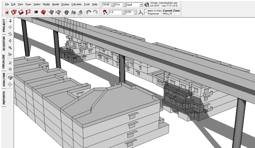
FIGURE 158: SHADOW RANGE ON 21<sup>ST</sup> APRIL 4 PM WITH VIADUCT
