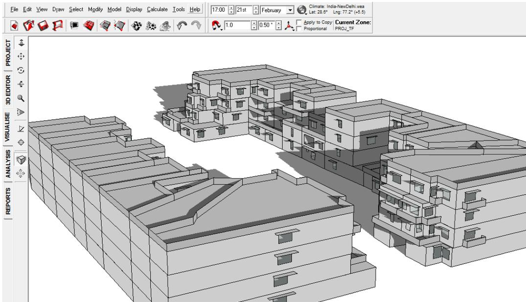
FIGURE 177: SHADOW RANGE ON 21<sup>ST</sup> FEBRUARY 5 PM WITHOUT VIADUCT
