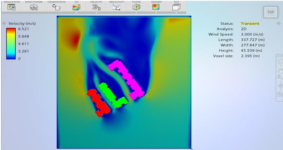
FIGURE 204: WIND ANALYSIS RESULT - WITHOUT VIADUCT
