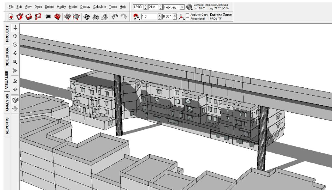
FIGURE 58: SHADOW RANGE ON 21<sup>ST</sup> FEBRUARY 12 PM WITH VIADUCT
