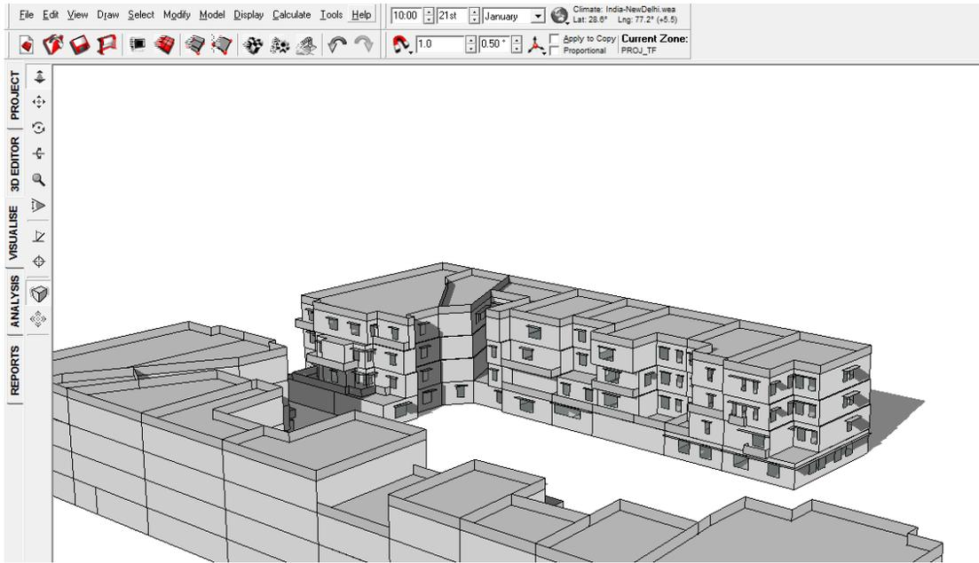
FIGURE 27: SHADOW RANGE ON 21<sup>ST</sup> JANUARY 10 AM WITHOUT VIADUCT
