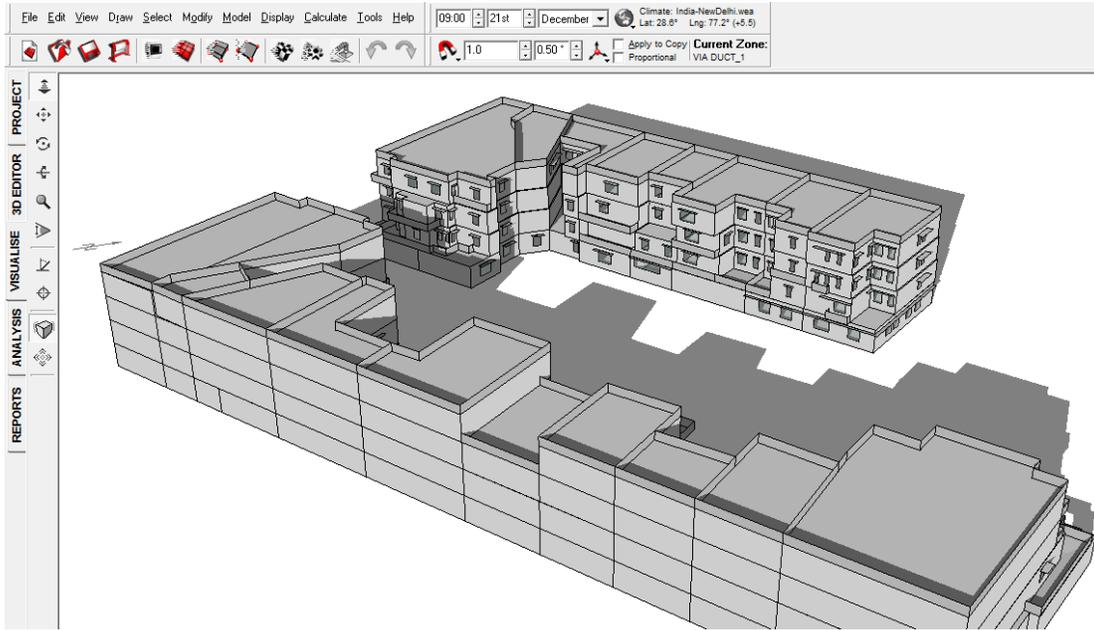
FIGURE 17: SHADOW RANGE ON 21<sup>ST</sup> DECEMBER 9 AM WITHOUT VIADUCT
