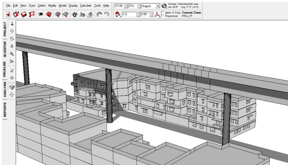
FIGURE 46: SHADOW RANGE ON 21<sup>ST</sup> AUGUST 11 AM WITH VIADUCT
