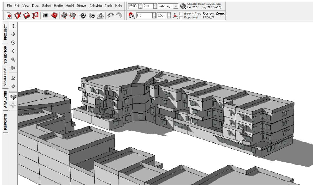
FIGURE 129: SHADOW RANGE ON 21<sup>ST</sup> FEBRUARY 3 PM WITHOUT VIADUCT
