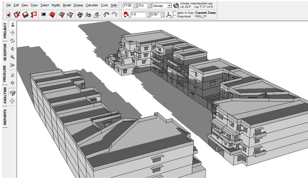
FIGURE 175: SHADOW RANGE ON 21<sup>ST</sup> JANUARY 5 PM WITHOUT VIADUCT
