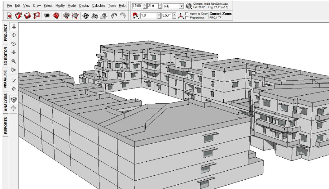
FIGURE 187: SHADOW RANGE ON 21<sup>ST</sup> JULY 5 PM WITHOUT VIADUCT
