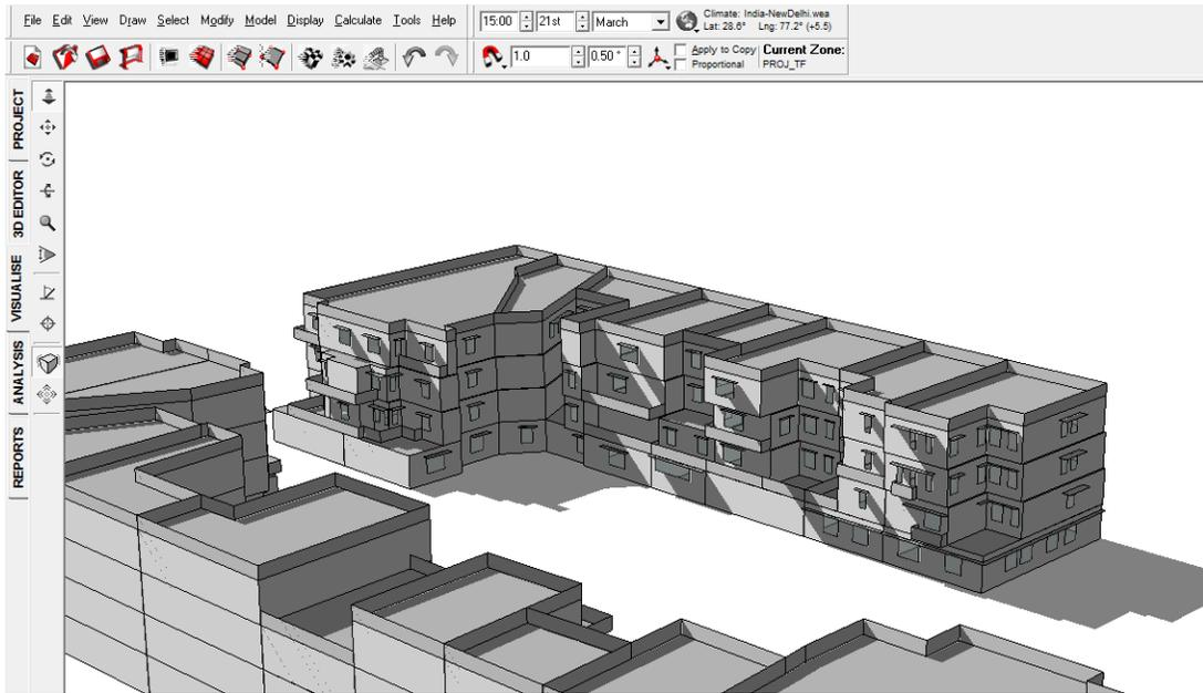
FIGURE 131: SHADOW RANGE ON 21<sup>ST</sup> MARCH 3 PM WITHOUT VIADUCT
