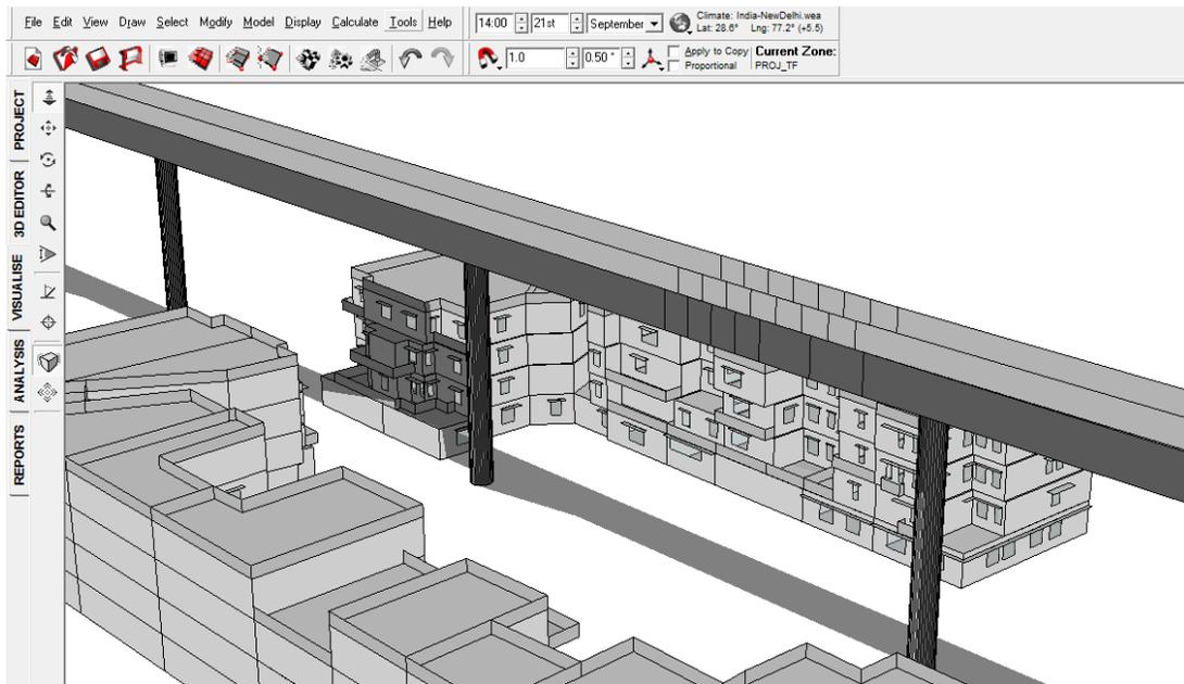
FIGURE 120: SHADOW RANGE ON 21<sup>ST</sup> SEPTEMBER 2 PM WITH VIADUCT
