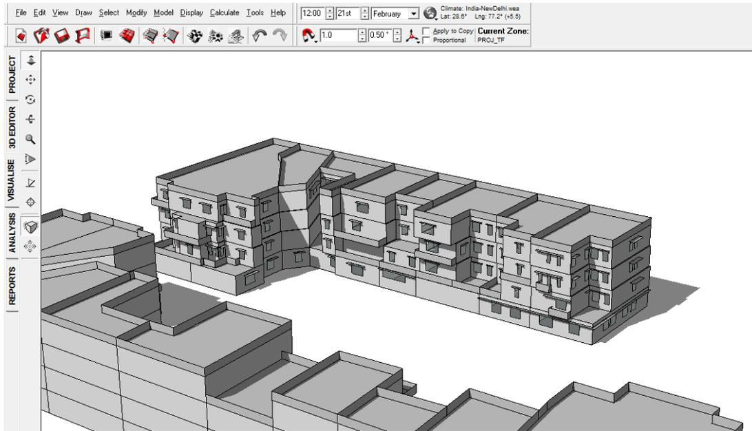
FIGURE 57: SHADOW RANGE ON 21<sup>ST</sup> FEBRUARY 12 PM WITHOUT VIADUCT
