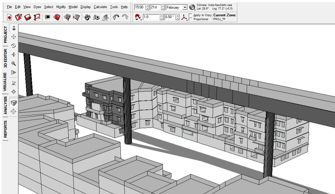
FIGURE 130: SHADOW RANGE ON 21<sup>ST</sup> FEBRUARY 3 PM WITH VIADUCT
